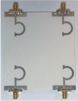
**Figure 3.** Photograph of multi-feed 4-elements planar antenna array.
