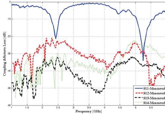
**Figure 7.** Measured mutual coupling results of the 4-elements planar antenna array system ( $2 \times 2$ ).
