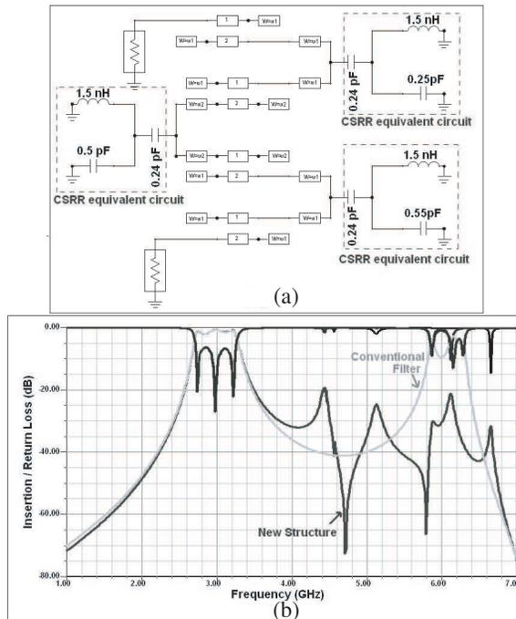
**Figure 4.** (a) Band pass hairpin filter schematic with three CSRRs coupled to deadlines. (b) Frequency response of filter with CSRRs ((a) schematic) compare whit conventional hairpin filter.
