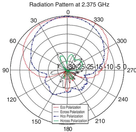
Figure 7. Measured radiation patterns for compact RDRA.
