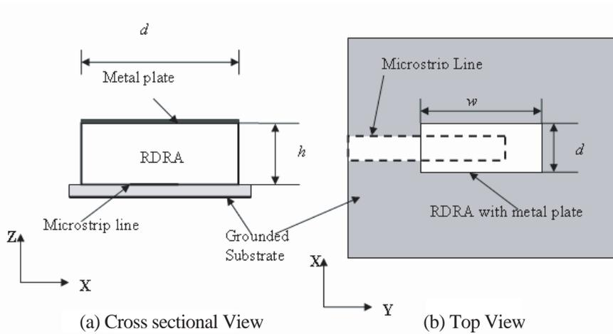
**Figure 3.** Geometry of the proposed compact RDRA.
