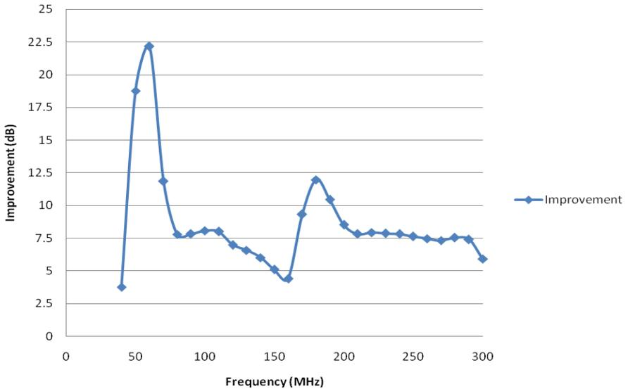
**Figure 4.** Value of improvement while replacing braided shield with adhesive foil.
