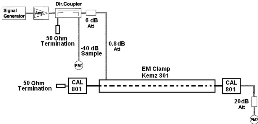
Figure 2. Block diagram of the measurement setup.
