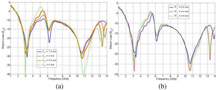
**Figure 5.** Simulated reflection coefficient curves for different (a) slot lengths  $L_S$  with  $W_S = 0.65$  mm and  $D_S = 18.6$  mm, (b) slot widths  $W_S$  with  $L_S = 8.6$  mm and  $D_S = 18.6$ .
