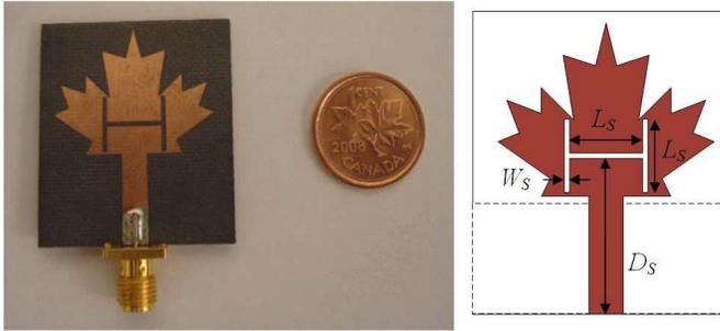
**Figure 4.** Geometry and photograph of the proposed bandstop antenna using an H-slot.
