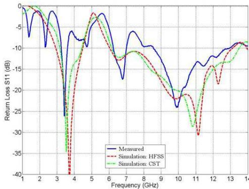
**Figure 6.** Measured and simulated reflection coefficient curves for the proposed bandstop antenna using an H-slot.
