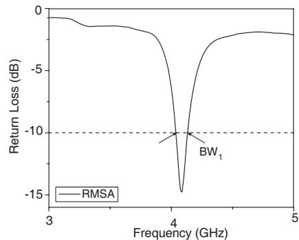
Figure 6. Variation of return loss versus frequency of RMSA.
