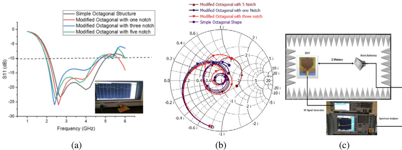
Figure 4. (a) Reflection coefficients of proposed antenna. (b) Smith Chart. (c) Measurement setup.
