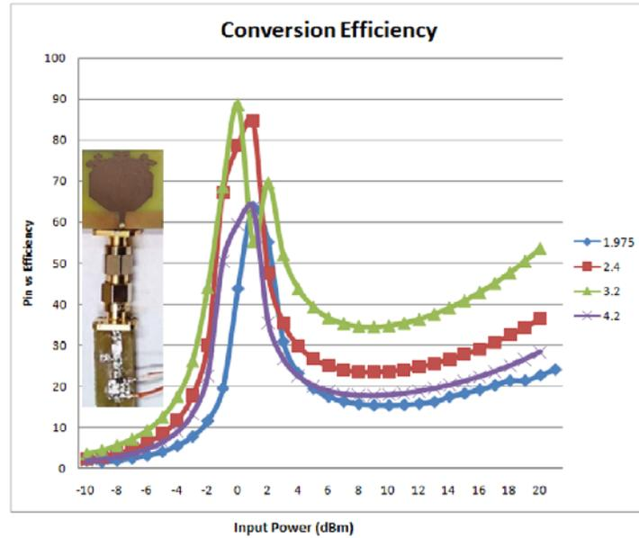
**Figure 5.** Power conversion efficiency of proposed rectenna.
