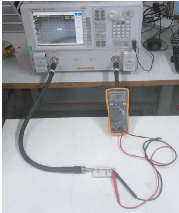
**Figure 17.** Photograph of output voltage measurement of the proposed rectifier at  $15\text{ dBm}$  input power received from E8363C PNA network analyzer considered as an RF source. (voltage =  $1.194\text{ V}$ ).
