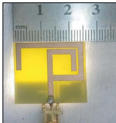
Figure 9. Prototype of proposed antenna.
