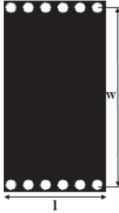
**Figure 3.** Layout of SIW structure.
