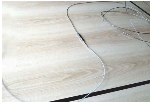
Figure 7. Typical cables used for OHDS system in an aircraft.
