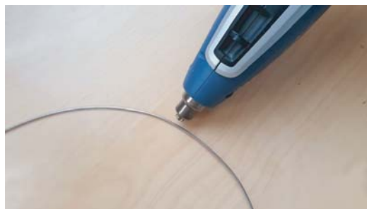
Figure 14. Heat-induced soft fault: hot spot in sensing element.
