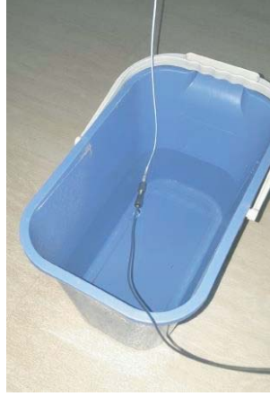
Figure 8. Water-induced soft fault — moisture in connectors.
