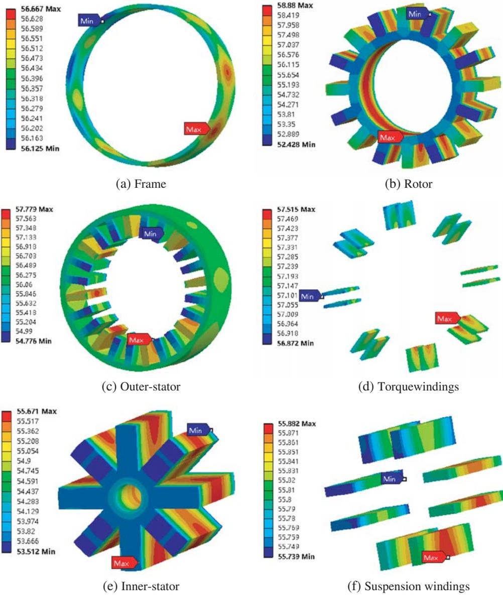
Figure 14. Temperature field distribution of the motor.
