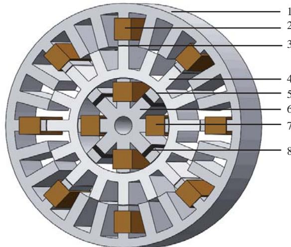
1-Outer stator; 2-Torque winding; 3-Air gap1; 4-Rotor;
