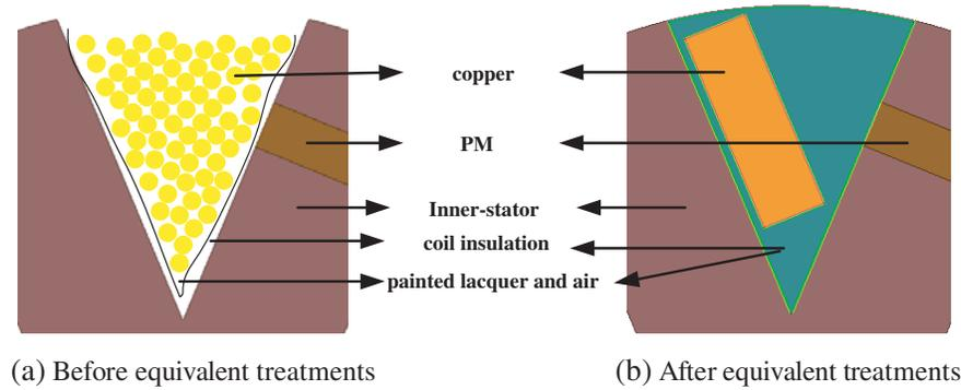
Figure 10. Equivalent treatment of suspension windings.
