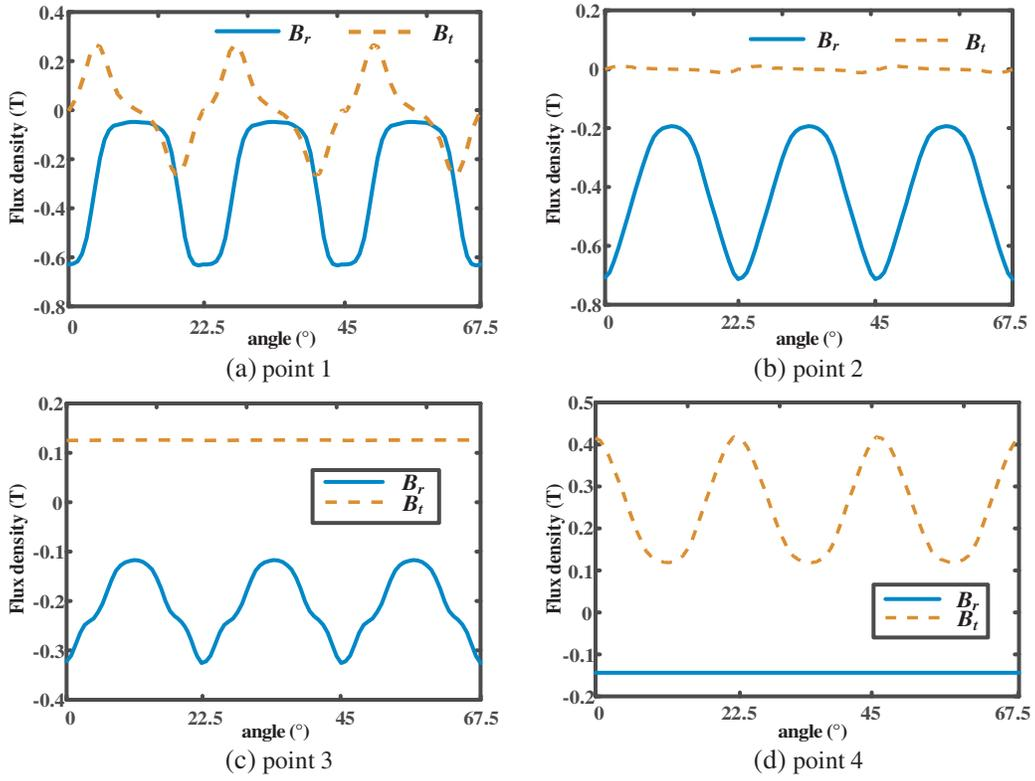
Figure 3. Magnetic density waveform on the outer-stator.
