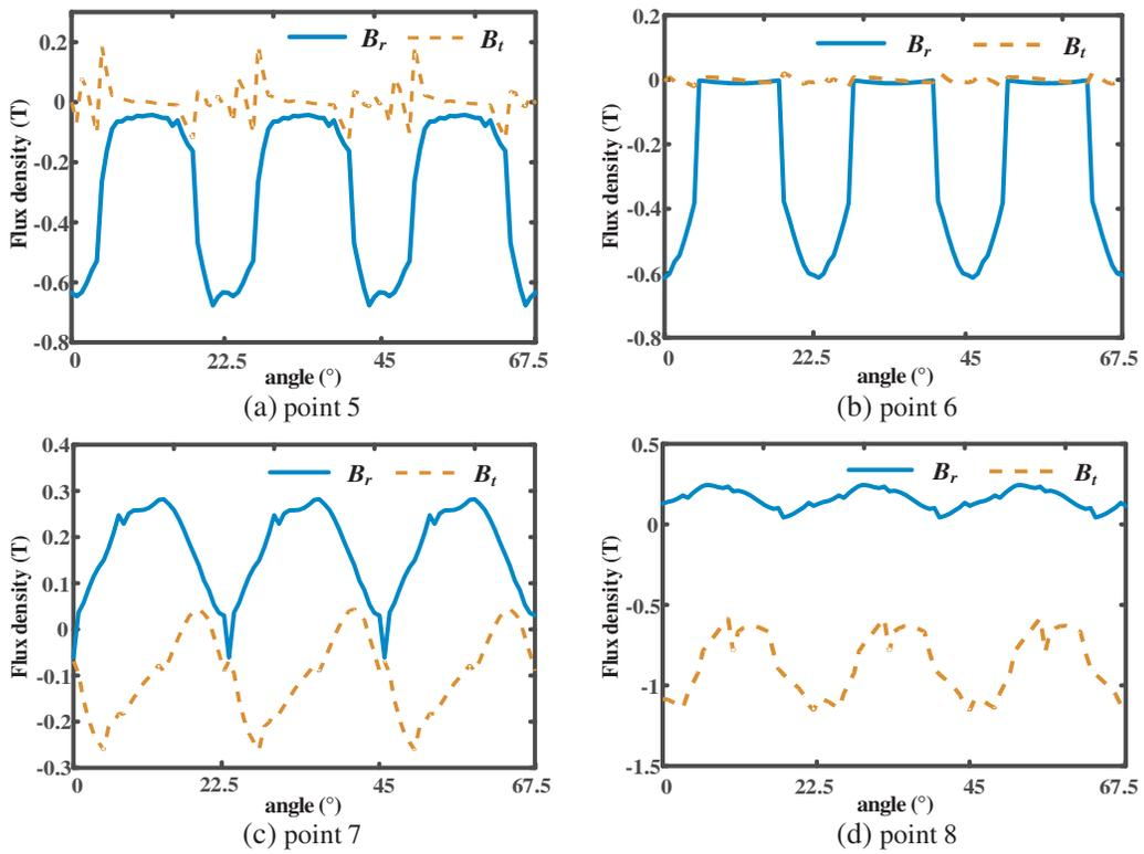
Figure 4. Magnetic density waveform on the rotor.
