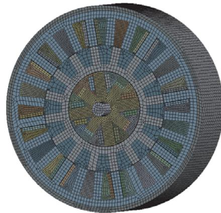
**Figure 11.** Thermal model of the HEDSBSRM.
