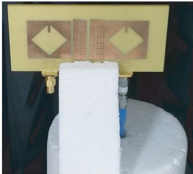
**Figure 5.** Radiation pattern measurement setup of the fabricated DLDP-EBG MIMO antenna.
