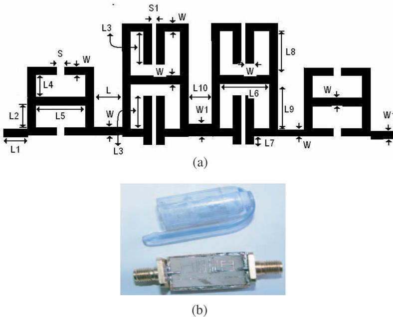
**Figure 4.** The layout of the proposed cascaded LPF with  $L = 0.88$  mm,  $L_1 = 2.2$  mm,  $L_2 = 2.5$  mm,  $L_3 = 1.5$  mm,  $L_4 = 1$  mm,  $L_5 = 3.2$  mm,  $L_6 = 1.98$  mm,  $L_7 = 0.5$  mm,  $L_8 = 1.8$  mm,  $L_9 = 2.5$  mm,  $L_{10} = 1.1$  mm,  $W = 0.3$  mm,  $W_1 = 0.69$  mm,  $S = 0.7$  mm, and  $S_1 = 0.38$  mm, (b) the fabricated of the proposed LPF.
