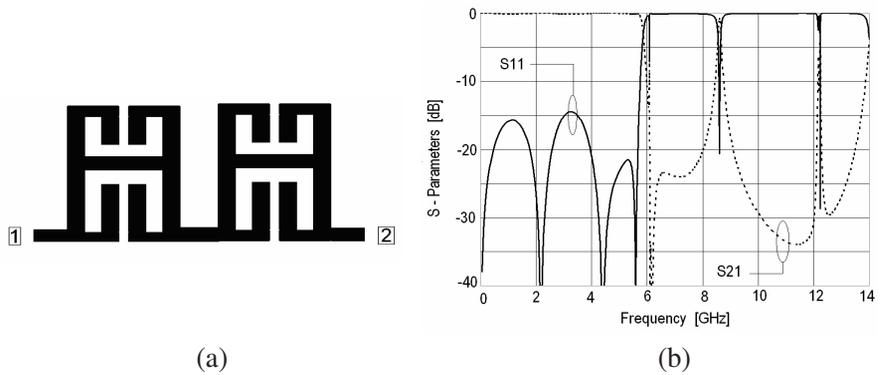
**Figure 3.** (a) the proposed LPF (b) its frequency response.
