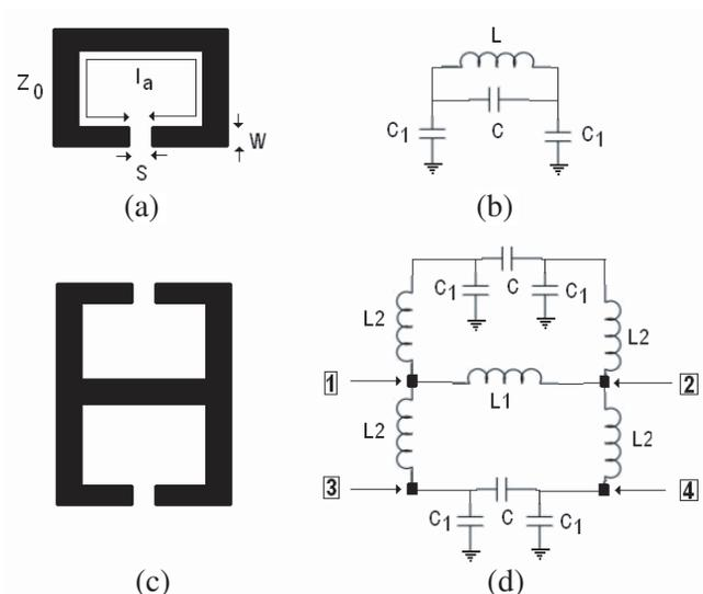
**Figure 1.** (a) and (b) the conventional microstrip open-loop resonator and its equivalent circuit model, (c) and (d) the proposed resonator and its equivalent circuit model.
