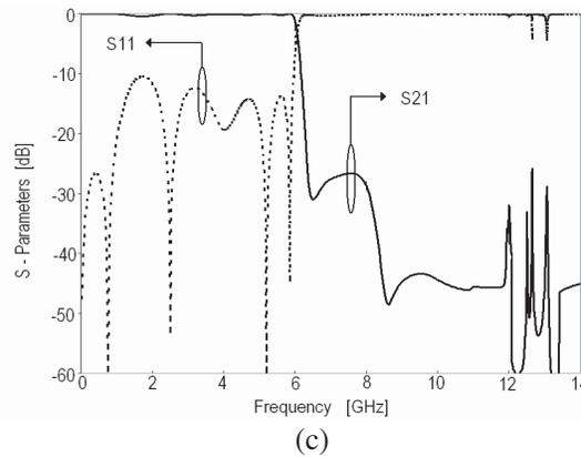
**Figure 5.** a)  $S_{21}$  within the 3-dB bandwidth for the proposed LPF (b) its simulated frequency response (c) measured results.
