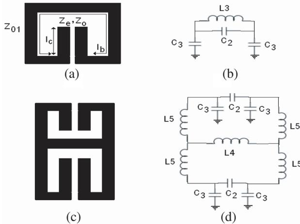
**Figure 2.** (a) and (b) the conventional microstrip semi-hairpin resonator and its equivalent circuit model, (c) and (d) the proposed resonator and its equivalent circuit model.
