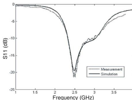
**Figure 7.** Reflection coefficient of the antenna shown in Fig. 4.
