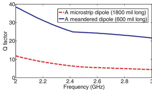
**Figure 3.** Q factor comparison of a miniaturized dipole (600 mils long) and a straight microstrip dipole (1800 mils long) with no bottom ground conductor.
