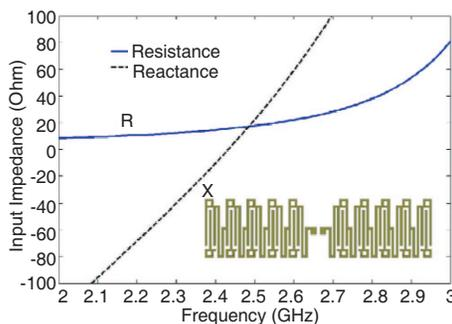
**Figure 2.** Input impedance of a meandered dipole antenna on a FR4 slab.
