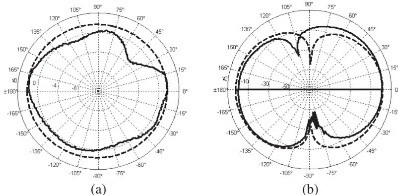
**Figure 8.** Simulated and measured radiation patterns. Dot-line: Simulation and solid line: measurement. (a)  $H$ -plane ( $x$ - $z$  plane in Fig. 4). (b)  $E$ -plane ( $y$ - $z$  plane in Fig. 4).
