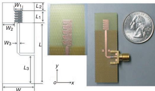
**Figure 4.** Miniaturized printed wire antenna on a FR4 substrate. Note that wire-and ground patch form a dipole.
