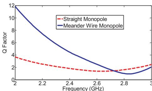
**Figure 9.** The Q factor of the designed miniaturized wire (300 mils long) in Fig. 4 and a straight microstrip monopole (900 mils long).
