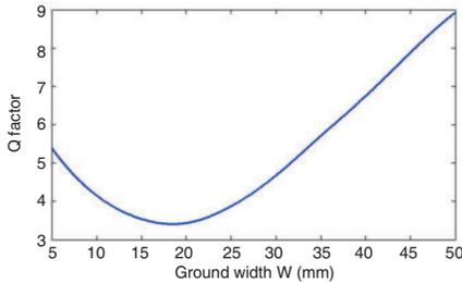
**Figure 5.** Q factor of the centered wire-patch antenna versus the ground width ( $W$ ) with  $L = 1500$  mils.
