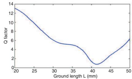
**Figure 6.** Q factor of the wire-patch antenna versus the ground length  $L$ . Other dimensions are given in Fig. 1 ( $W = 666$  mils).
