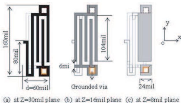
**Figure 1.** The drawing of a unit cell in the meandered dipole. Note that for antenna application, the ground plane at  $z = 0$  is partially removed.
