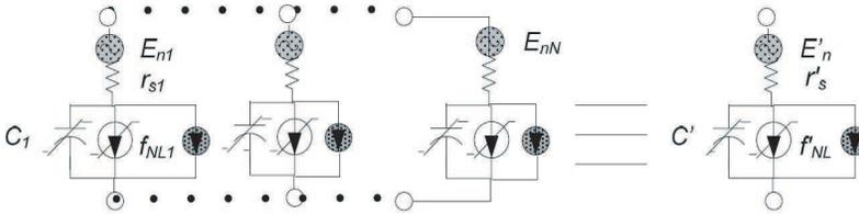
**Figure 4.** Equivalent diode model for N APDP(s).
