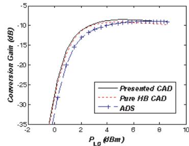
**Figure 7.** Conversion gain calculated in three ways.
