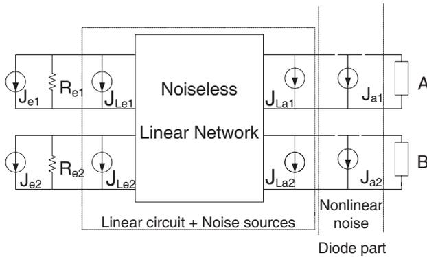
**Figure 5.** The circuit presentation for the small signal and noise analysis.
