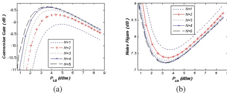
Figure 8. (a) Conversion gain for  $N$  APDP(s), (b) noise figure for  $N$  APDP(s).
