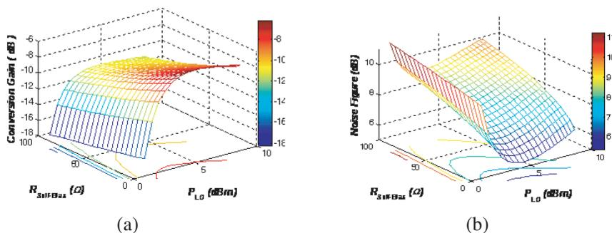
Figure 9. (a) Conversion gain and (b) noise figure versus self-biased and  $P_{LO}$ .
