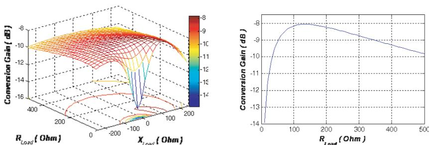
Figure 10. Conversion gain for swap  $Z_{Load} = R_{Load} + jX_{Load}$ .
