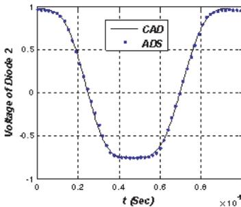
**Figure 6.** Steady state large signal voltage of nonlinear port.
