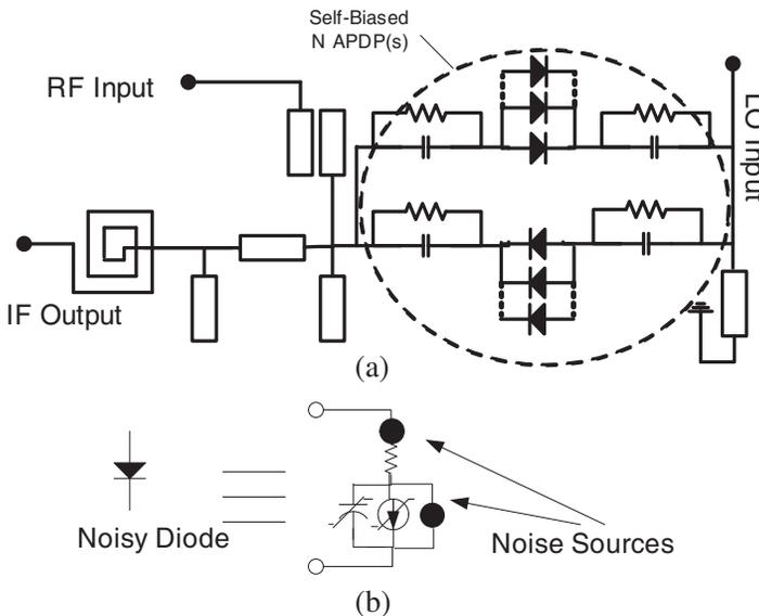
**Figure 1.** (a) Mixer structure, (b) nonlinear noisy diode model.
