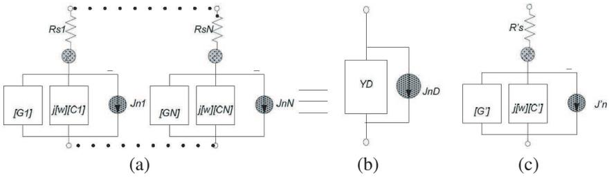
**Figure 3.** Equivalent diode part for simultaneous signal and noise analysis.
