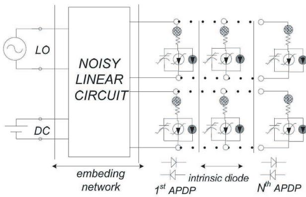
**Figure 2.** The circuit presentation for the steady state response in simultaneous signal and noise analysis based on HB nonlinear analysis.
