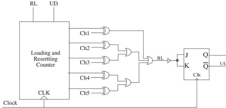
**Figure 6.** Architecture of fully-integrated pulse-swallow counter.
