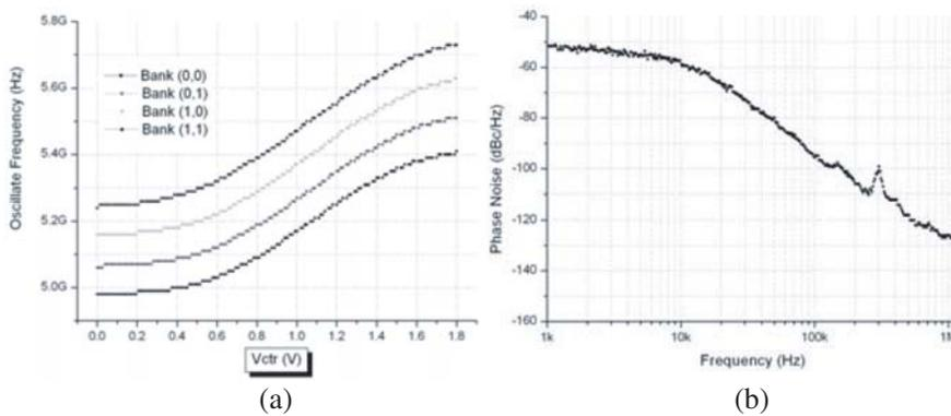
Figure 11. (a) Measured tuning range under different banks; (b) Phase noise is  $-126$  dBc/Hz@1 MHz offset.
