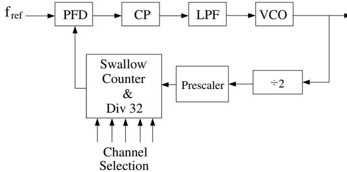
**Figure 1.** Basic architecture of an integer-N frequency synthesizer.
