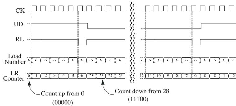
**Figure 7.** Analysis of a pulse-swallow counter.
