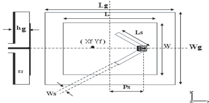
**Figure 1.** The geometry of a patch antenna with a switchable V-slot (PASVS).
