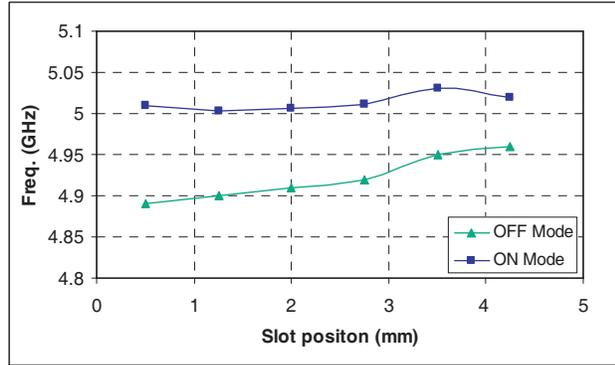
**Figure 8.** The resonant frequency of the PASVS (CST simulation) the slot position.
