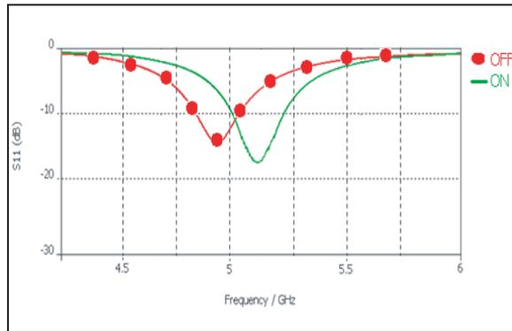
**Figure 13.** The measured  $S_{11}$  comparison for both of the OFF and ON switch modes for the fabricated antenna. The frequency ratio was 1.078.
