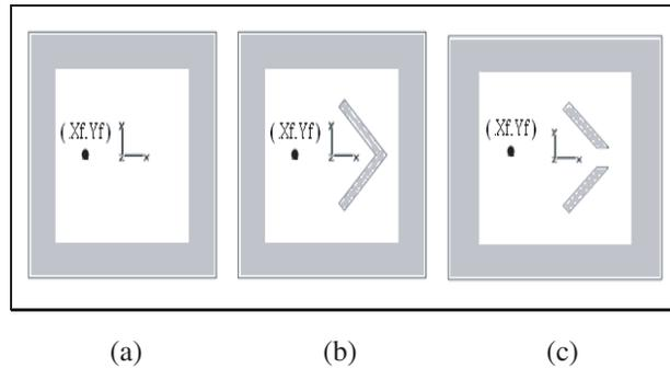
**Figure 2.** (a) The patch antenna without slot, (b) OFF mode, (c) ON mode.
