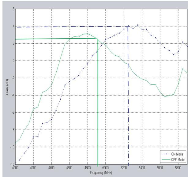
**Figure 14.** The measured total gain radiation pattern for both of the OFF and ON switch modes for the fabricated antenna.
