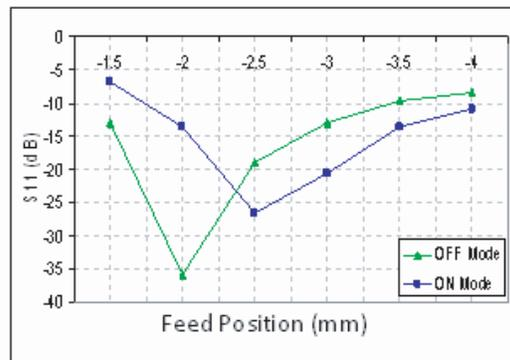
**Figure 4.** The effect of the different feeding positions on the return loss of the PASVS antenna.
