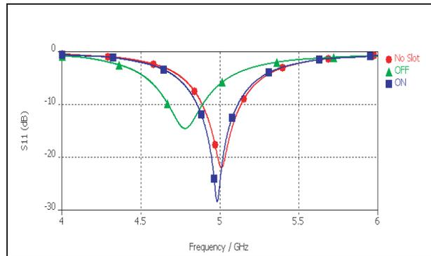
**Figure 9.** The CST-simulated  $S_{11}$  results of a PASVS for the ON/OFF modes of the switch, compared to a patch antenna without a slot. The frequency ratio of the two modes was 1.05.
