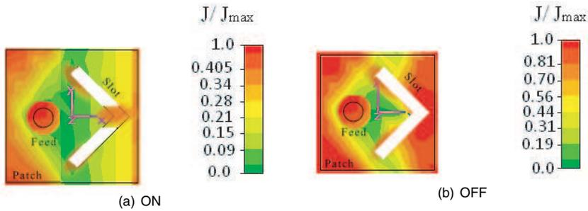
**Figure 15.** The normalized electric current densities (normalized to the maximum current  $J_{\max}$  in the patch) on the patch at the resonant frequency for each of the two cases: (a) ON mode, (b) OFF mode.
