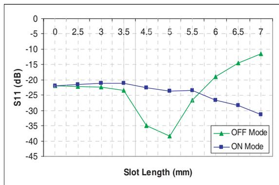
Figure 6.  $S_{11}$  versus the slot length.
