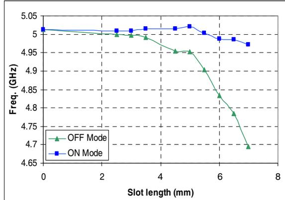
**Figure 5.** The simulated resonant frequency of the PASVS versus the slot length.
