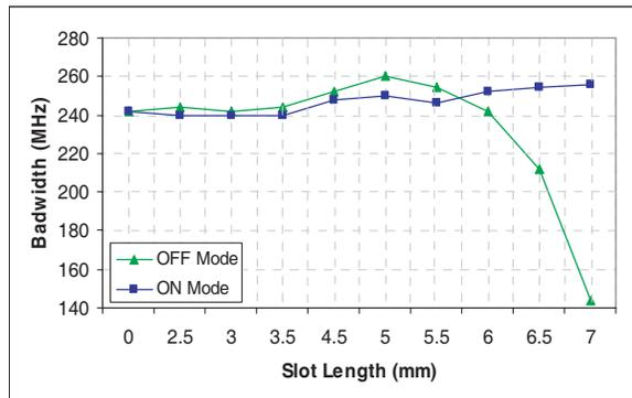
Figure 7. Bandwidth versus the slot length.
