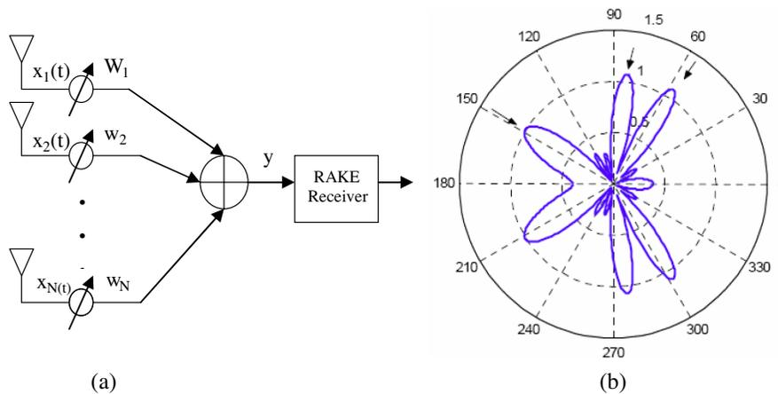
**Figure 1.** Beamforming (a) Beamformer principle for frequency selective channels (b) The beamforming characteristic of the multi-path MVDR algorithm for a single user.
