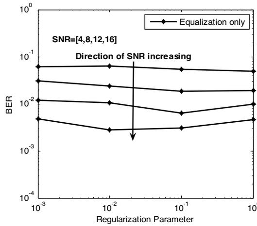
Figure 4. BER vs. regularization parameter at different SNR values for the equalization algorithm only.
