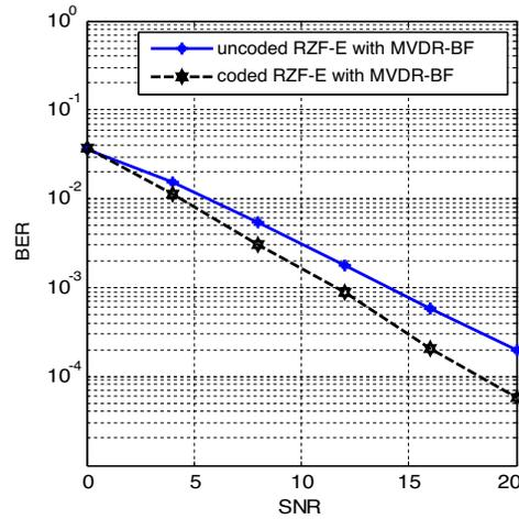
**Figure 7.** BER vs. SNR for uncoded and coded versions of the proposed scheme.
