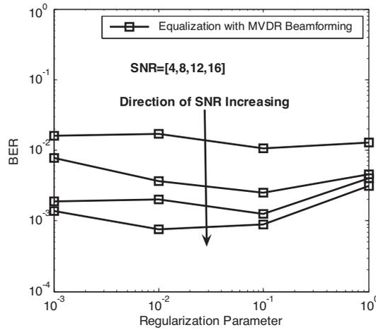
Figure 5. BER vs. regularization parameter at different SNR for the equalization with MVDR beam forming algorithm.
