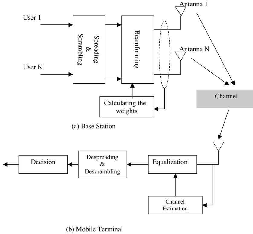
**Figure 2.** The proposed scheme (a) Transmitter (Base station) (b) Receiver (Mobile terminal).
