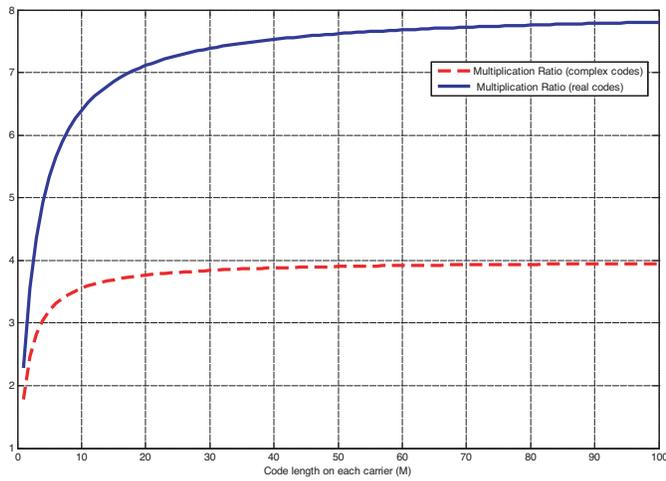
**Figure 11.** Computational load ratio of conventional and FFT based methods versus code length ( $f_s = 4P/t_c$ ,  $P = 4$ ).
