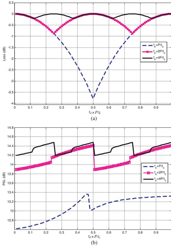
**Figure 3.** (a) Compression loss versus normalized target delay ( $t_d/t_s$ ) for 3 sampling frequencies ( $M = P = 5$ , Target delay =  $9.1t_c$ , and  $t_s = t_c/P$ ). (b) The ratio of the peak power to maximum sidelobe level versus normalized target delay ( $t_d/t_s$ ) for 3 sampling frequencies ( $M = P = 5$ , Target delay =  $9.1t_c$ , and  $t_s = t_c/P$ ).
