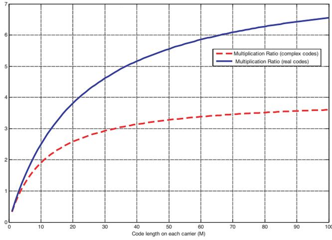
**Figure 10.** Computational load ratio of conventional and DFT based methods versus code length ( $f_s = 4P/t_c$ ,  $P = 5$ ).
