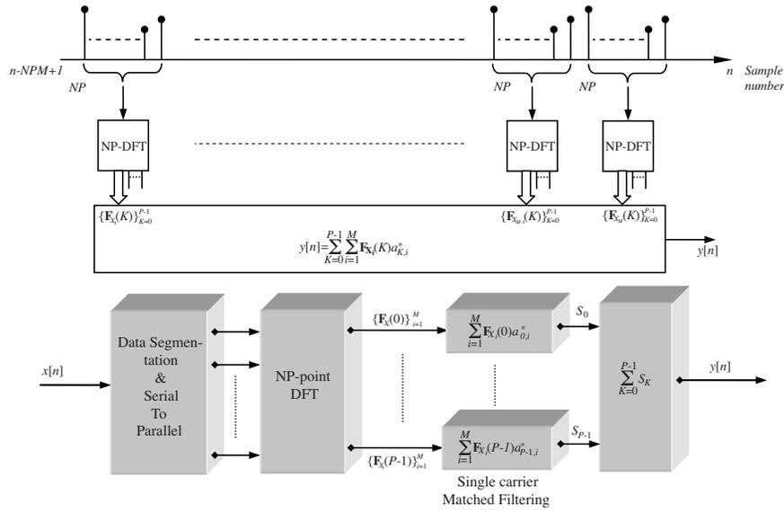
**Figure 2.** Block diagram of the proposed method to compress the MCPC signals.
