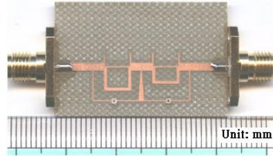
**Figure 6.** Photograph of a fabricated broadband bandpass filter.
