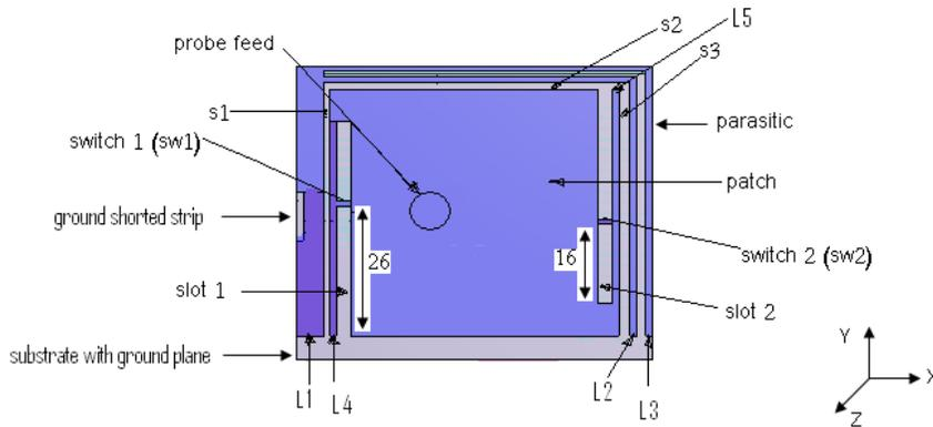
**Figure 1.** The Geometry and parameters of the proposed antenna.
