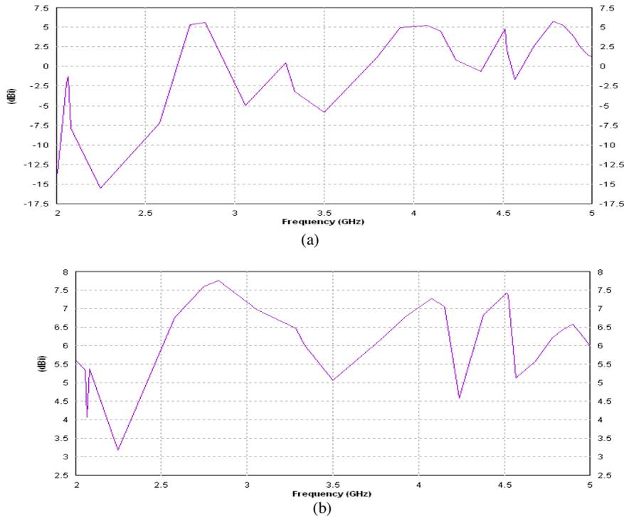
**Figure 5.** Behaviors of the gain (a) and directivity (b) of the proposed antenna as a function of frequency.
