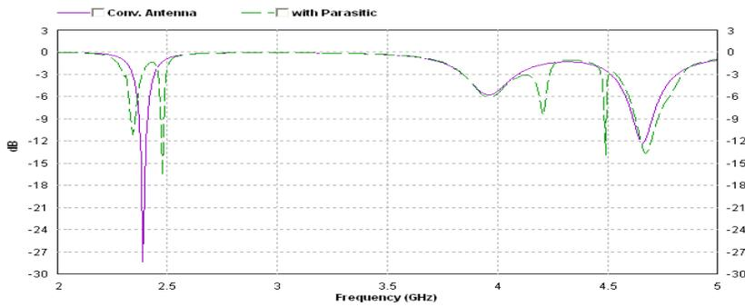
**Figure 2.** Return loss as a function of frequency for the conventional antenna and the conventional antenna with the parasitic.
