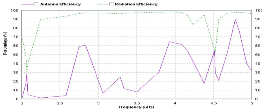
**Figure 6.** Behaviors of the antenna and radiation efficiencies of the proposed antenna with frequency.
