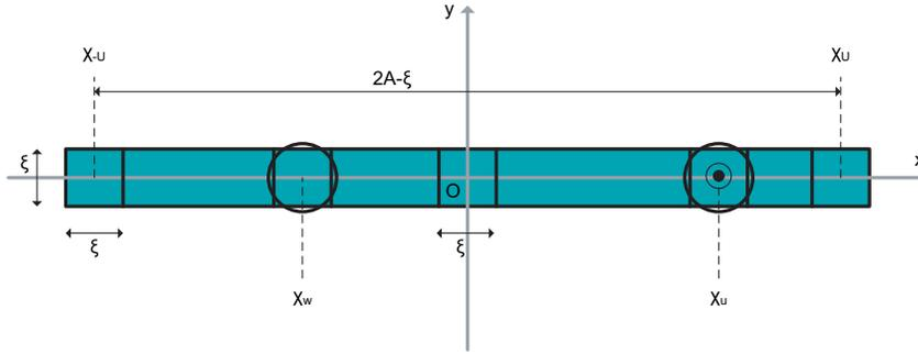
**Figure 2.** The approximate integration procedure on each pixel. Every square portion comprising the strip is replaced by a circle of equal area.
