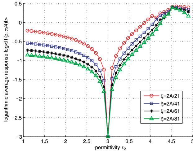
**Figure 4.** The average response of the device  $\log \langle |T(\phi, \Theta)| \rangle$  as function of the strip permittivity  $\epsilon_2$  for various thicknesses of the strip  $\xi$ . Plot parameters:  $\Theta = \pi/4$ ,  $A = \lambda_0$ ,  $\epsilon_1 = 3$ .
