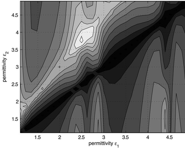
**Figure 5.** The backward response of the device  $|T(\Theta, \Theta)|$  in contour plot as function of the permittivities  $(\epsilon_1, \epsilon_2)$ . Plot parameters:  $\Theta = \pi/2$ ,  $A = \lambda_0$ ,  $\xi = 2A/51$ .
