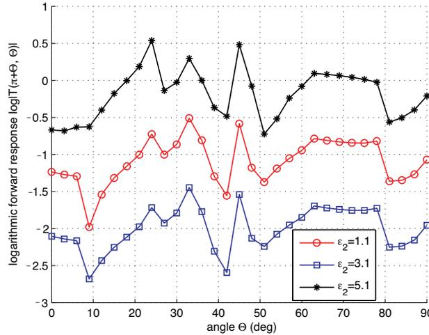
**Figure 3.** The forward response of the device  $\log |T(\pi + \Theta, \Theta)|$  as function of the incidence angle  $\Theta$  for various strip permittivities  $\epsilon_2$ . Plot parameters:  $A = \lambda_0$ ,  $\epsilon_1 = 3$ ,  $\xi = 2A/51$ .
