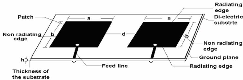
Figure 2.  $H$ -plane coupled rectangular microstrip antenna.
