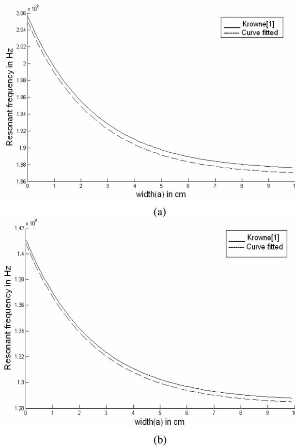
**Figure 6.** Resonant frequency versus width plot for (a)  $\epsilon_r = 2.5$  (b)  $\epsilon_r = 5$  of a  $H$ -plane mutually coupled rectangular microstrip patches for  $f_{design} = 3$  GHz,  $d/\lambda = 0.1$ ,  $h = 3048$  cm and  $b = 5$  cm.
