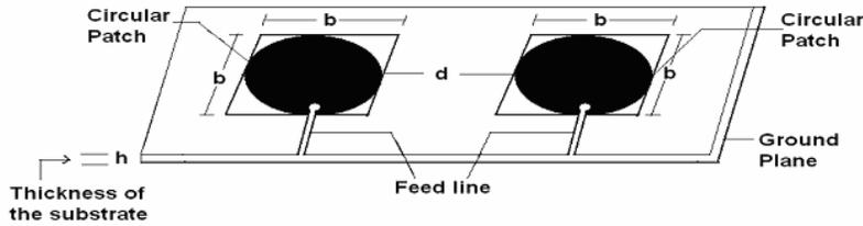
**Figure 3.** Mutually coupled equivalent circular microstrip antenna.
