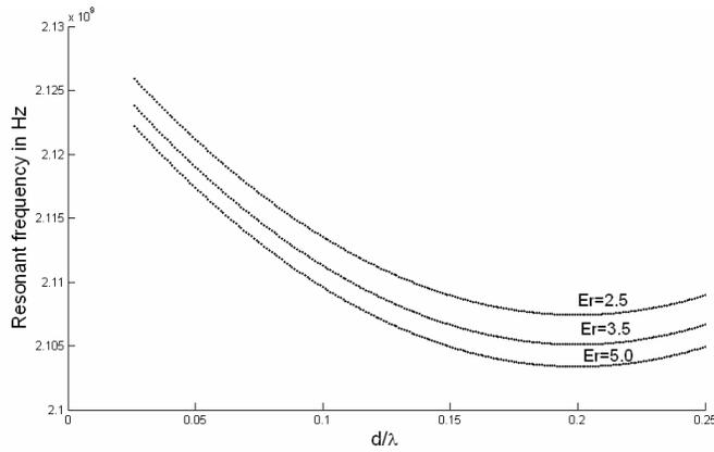
**Figure 5.** Resonant frequency versus  $d/\lambda$  plot for various  $E_r (= \epsilon_r)$  of  $H$ -plane coupled circular microstrip patches for  $f_{design} = 3\text{ GHz}$ ,  $h = 3048\text{ cm}$  and  $a = b = 5\text{ cm}$ .
