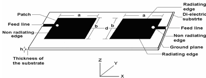
Figure 1.  $E$ -plane coupled rectangular microstrip antenna.
