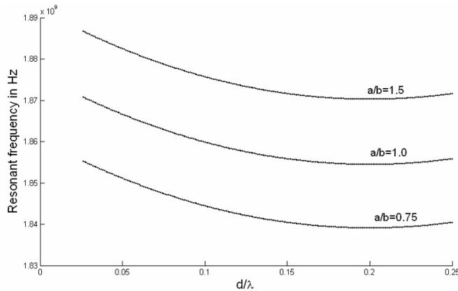
**Figure 4.** Resonant frequency versus  $d/\lambda$  plot of  $H$ -plane coupled rectangular microstrip patches for  $\epsilon_r = 2.5$ ,  $f_{design} = 3\text{ GHz}$ ,  $h = 3048\text{ cm}$  and  $b = 5\text{ cm}$ .
