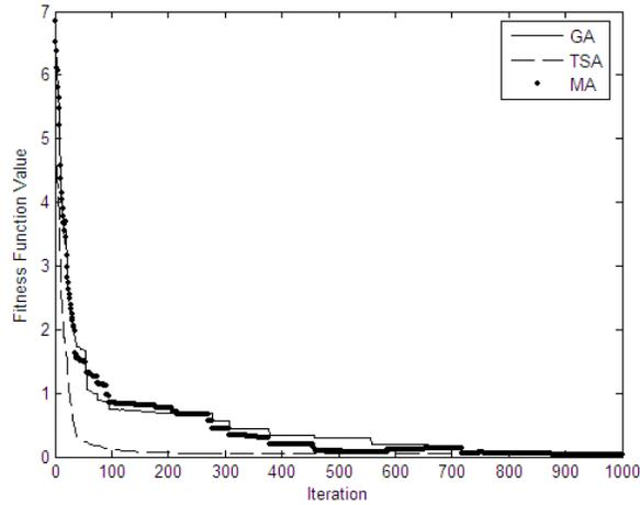
**Figure 6.** Convergence curve of the fitness value of the 26 element linear array versus the number of iterations. The GA, TSA and MA are attempting to reach the minimum value of the fitness function.
