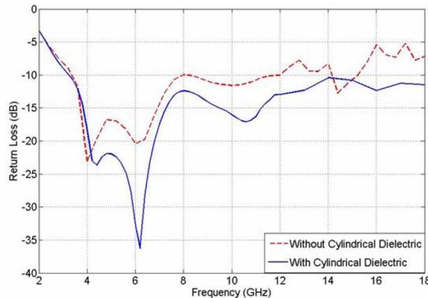
**Figure 7.** Simulated return loss of the proposed antenna with and without dielectric.  $2a = 19.5$  mm,  $2b = 31.4$  mm,  $l = 7.1$  mm,  $W = 2$  mm,  $R = 46$  mm,  $h = 2.3$  mm,  $r = 2.6$  mm and  $\alpha = 45^\circ$ .
