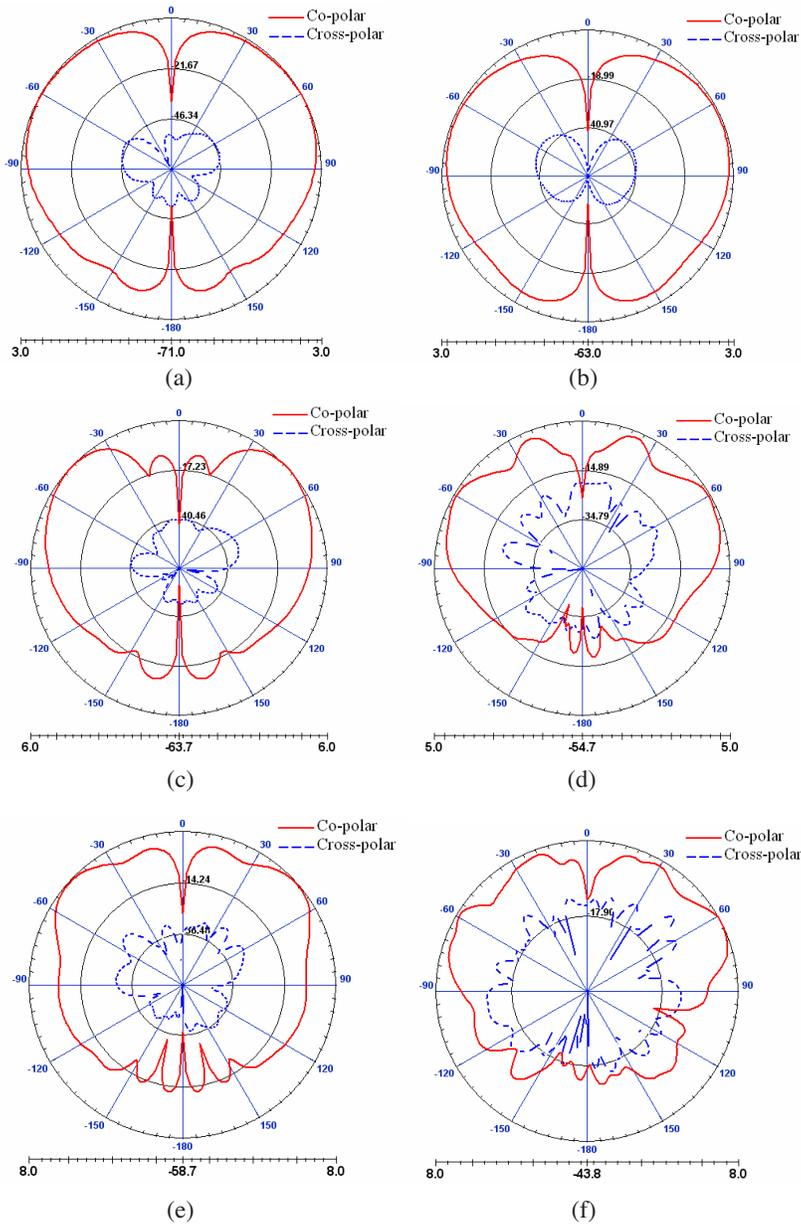
**Figure 3.** Simulated radiation patterns at: 3 GHz in (a)  $x-z$  plane, (b)  $y-z$  plane, 10 GHz in (c)  $x-z$  plane (d)  $y-z$  plane, 18 GHz in (e)  $x-z$  plane, (f)  $y-z$  plane.  $2a = 19.5$  mm,  $2b = 31.4$  mm,  $l = 7.1$  mm,  $W = 2$  mm,  $R = 46$  mm,  $h = 2.3$  mm,  $r = 2.6$  mm and  $\alpha = 45^\circ$ .
