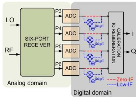
**Figure 16.** Block diagram of the dual zero-IF/low-IF six-port receiver.
