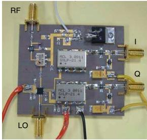
**Figure 9.** Fabricated zero-IF/low-IF receiver prototype.
