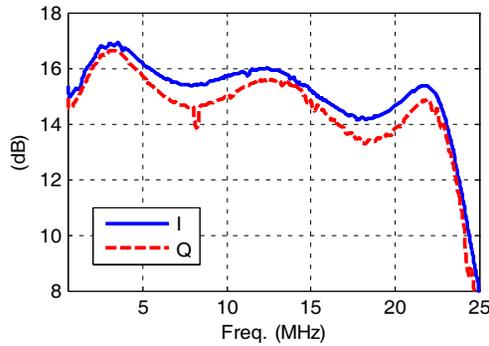
**Figure 13.** Measured IF response of the zero-IF/low-IF receiver.
