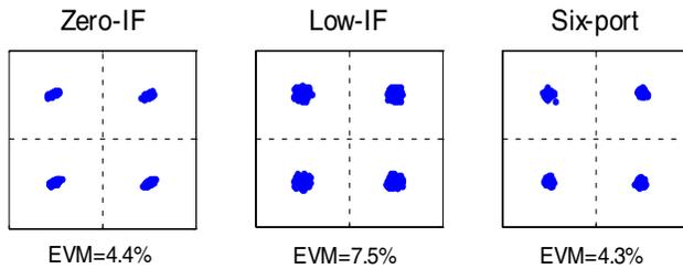
**Figure 14.** Constellation diagrams: 2595 MHz, 25 Mbps QPSK,  $P_{in} = -25$  dBm,  $P_{LO} = 0$  dBm.
