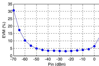
**Figure 19.** LTCC six-port receiver performance: measured EVM versus Pin at 2.5 GHz, 75 Mbps 6-QAM,  $P_{LO} = 0$  dBm.
