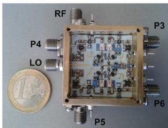
**Figure 18.** Fabricated  $30 \times 30 \times 1.25$  mm 0.3–6 GHz LTCC six-port receiver.
