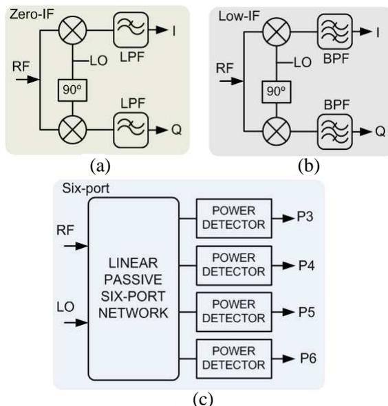
**Figure 1.** RF architectures for SDR (a) zero-IF, (b) low-IF, (c) six-port.
