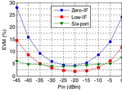
**Figure 11.** Measured EVM versus  $P_{in}$ : 2595 MHz, 30 Mbps 64-QAM,  $P_{LO} = 0$  dBm.
