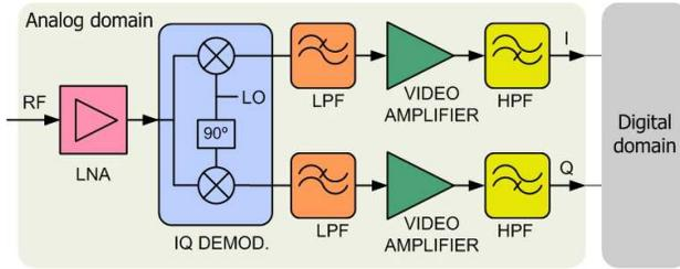
**Figure 8.** Block diagram of the zero-IF/low-IF receiver.
