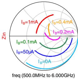
**Figure 6.** HSMS-286 diode input impedance.
