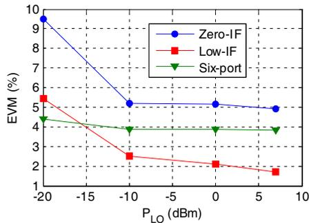
**Figure 15.** Measured EVM versus  $P_{LO}$ : 2595 MHz, 10 Mbps QPSK,  $P_{in} = -20$  dBm.
