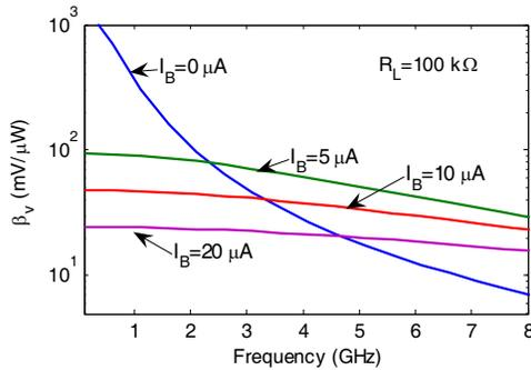
**Figure 5.** Theoretical detector diode voltage sensitivity, HSMS-286B.
