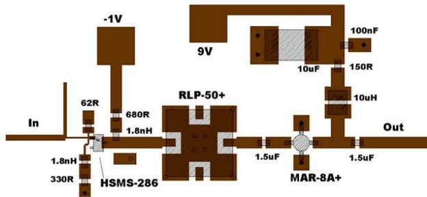
**Figure 7.** Layout of the circuit composed of the detector diode and the baseband components.
