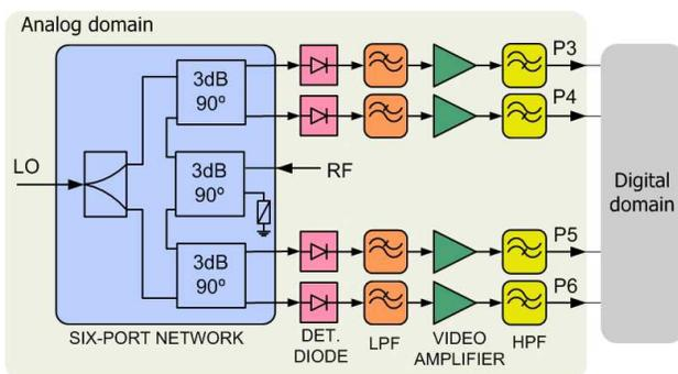
**Figure 2.** Block diagram of the six-port receiver.
