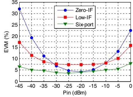
**Figure 12.** Measured EVM versus  $P_{in}$ : 2595 MHz, 75 Mbps 64-QAM,  $P_{LO} = 0$  dBm.
