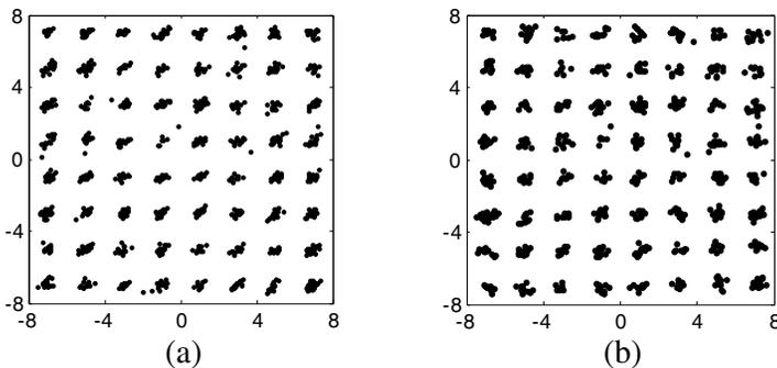
**Figure 17.** Constellation diagrams obtained from the six-port receiver in (a) low-IF and (b) zero-IF operation modes.
