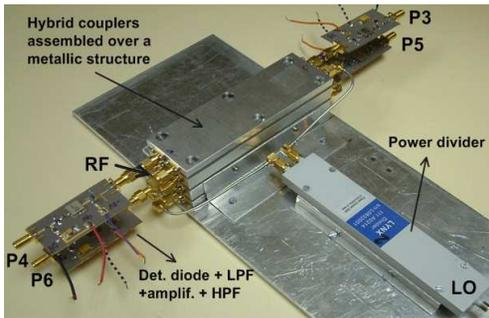
**Figure 3.** Fabricated six-port receiver prototype.
