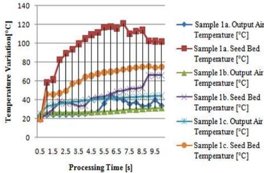
**Figure 9.** Temperature variation in constant heating using 0.3 W/g.
