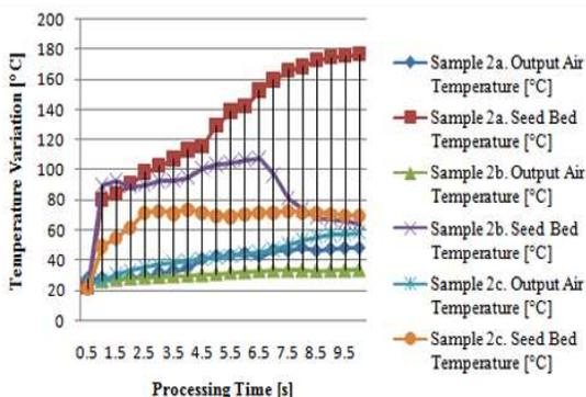
Figure 12. Temperature variation in constant heating using 0.4 W/g.
