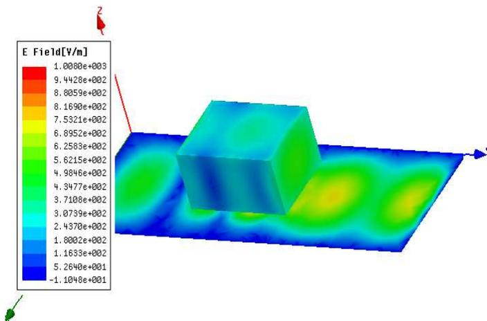
**Figure 2.** Electric field distribution over the base plan of the cavity and dielectric.
