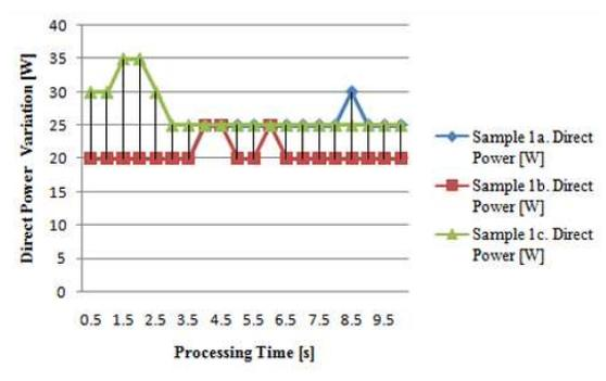
Figure 8. Direct power variation in constant heating using 0.3 W/g.
