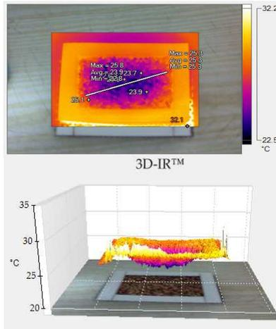
**Figure 14.** Temperature distribution over the seed bed and the 3D distribution of the temperature of the witness sample.
