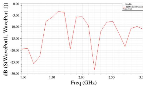
**Figure 5.** Reflected power to the magnetron expressed through the  $S$  parameters, in dB.
