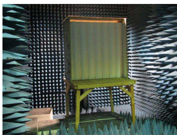
Figure 10. All-dielectric FSS with few periods setup inside an anechoic chamber.
