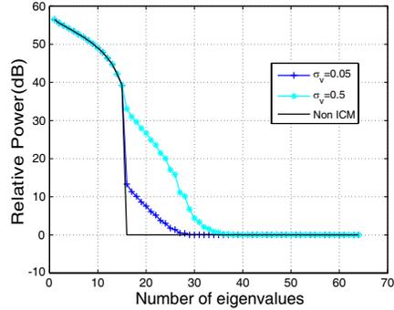
**Figure 5.** Clutter eigenspectrum with different ICM.
