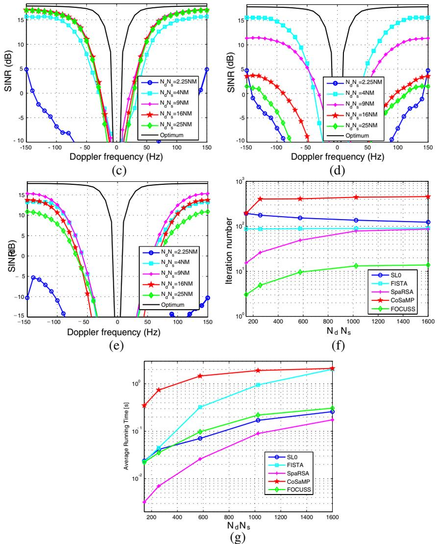
**Figure 1.** Impacts of sizes of dictionary on SINR performance against Doppler frequency with 6 snapshots and target Doppler frequency space from  $-150\text{ Hz}$  to  $150\text{ Hz}$ . (a) SL0. (b) FISTA. (c) SpaRSA. (d) CoSaMP. (e) FOCUSS. (f) Iteration number versus sizes of dictionary for all algorithms. (g) Average running time versus sizes of dictionary for estimating one angle-Doppler profile.
