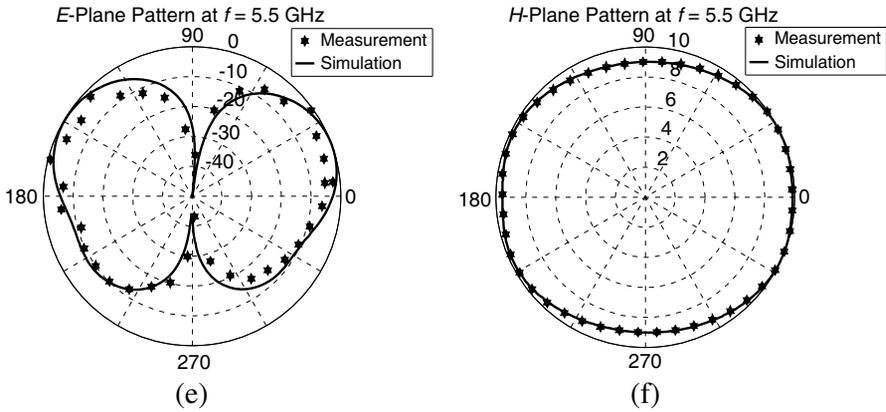
**Figure 14.** Normalized patterns of wideband PTM antenna for WLAN. At 2.4 GHz: (a) *E*-plane (*xoz*); (b) *H*-plane (*yoz*). At 4 GHz: (c) *E*-plane (*xoz*); (d) *H*-plane (*yoz*). At 5.5 GHz: (e) *E*-plane (*xoz*); (f) *H*-plane (*yoz*).
