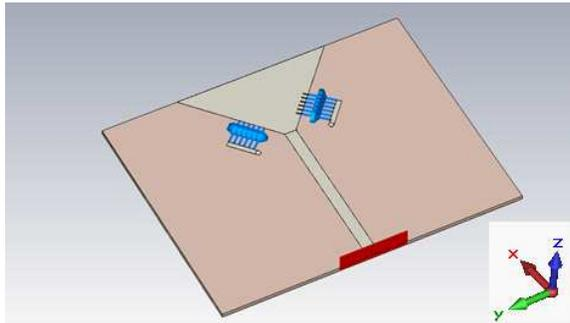
**Figure 7.** Replacement of combline stub loading by appropriate lumped inductors.
