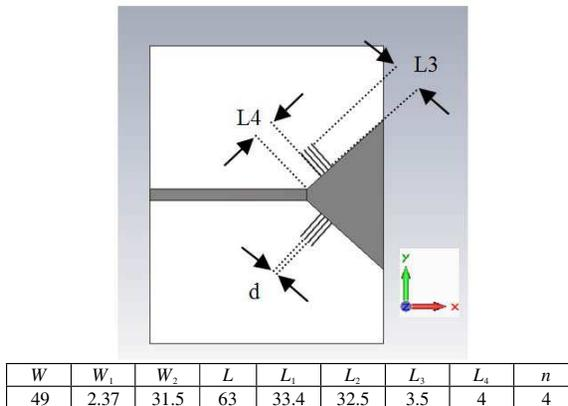
**Figure 4.** Loaded PTM antenna. Dimensions are in millimeters.
