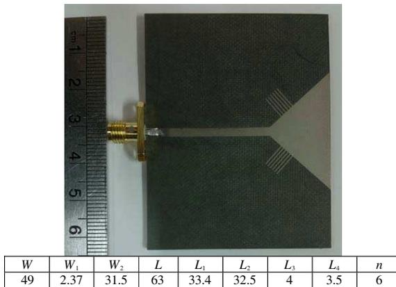
**Figure 13.** Fabricated prototype of wideband PTM antenna. Dimensions are in millimeters.
