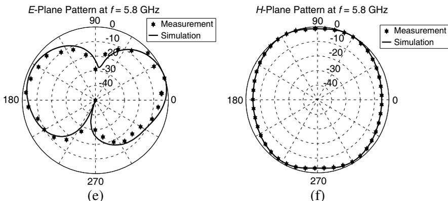
**Figure 10.** Normalized patterns of loaded PTM antenna for WLAN. At 2.4 GHz: (a) *E*-plane (*xoz*); (b) *H*-plane (*yo<sub>z</sub>*). At 5 GHz: (c) *E*-plane (*xoz*); (d) *H*-plane (*yo<sub>z</sub>*). At 5.8 GHz: (e) *E*-plane (*xoz*); (f) *H*-plane (*yo<sub>z</sub>*).
