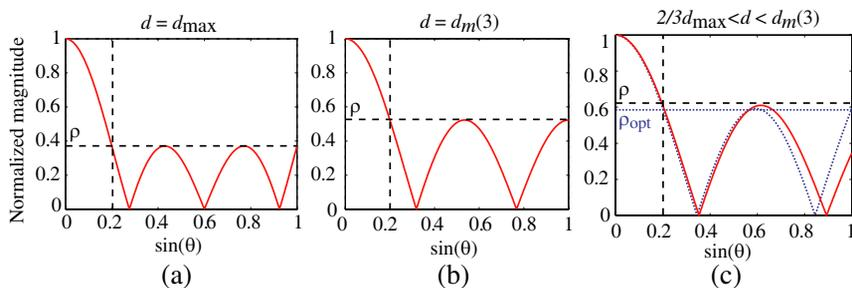
**Figure 2.** Far field patterns of a four element linear array of diminishing length  $3d$  synthesized by the Dolph Chebyshev method, where  $\sin \theta_s = 0.2$ . As  $d$  decreases,  $\rho$  increases. In (c), the optimal pattern which, in this case, is different from the DC pattern, is added in dotted line.
