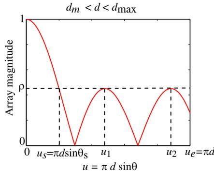
**Figure 3.** Far field pattern of a four element linear array synthesized by the Dolph Chebyshev method with some useful notations.
