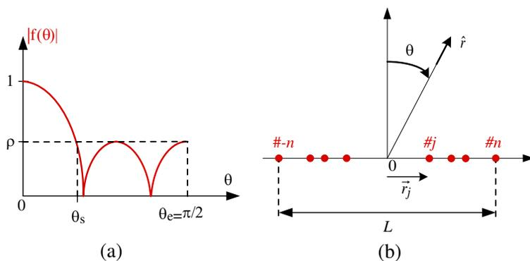
**Figure 1.** (a) Schematic view of the pattern synthesis problem. The magnitude of the far field pattern  $|f(\theta)|$  is normalized to unity in the broadside direction ( $|f(0)|=1$ ) whereas one minimizes its sidelobe level  $\rho$  for a fixed half beam width  $\theta_s$ . (b) Geometry of the linear array of length  $L$  composed of  $N$  isotropic elements. The observation angle  $\theta = 0$  corresponds to the broadside direction.
