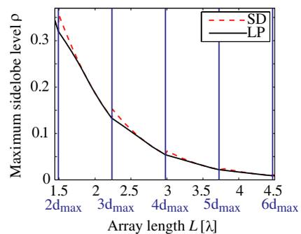
**Figure 5.** Maximum sidelobe level as a function of the array length for a half beam width  $\theta_s$  of  $20^\circ$ . The results applying the *sparsest* Dolph design (SD) and the optimal array obtained by LP are compared for  $L$  ranging between  $2d_{\max}$  and  $6d_{\max}$ .
