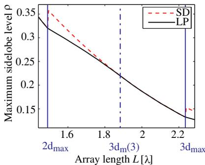
**Figure 4.** Maximum sidelobe level as a function of the array length for a half beam width  $\theta_s$  of  $20^\circ$ . The results applying the *sparsest* Dolph design (SD) and the optimal array obtained by LP are compared for  $L$  ranging between  $2d_{\max}$  and  $3d_{\max}$ . They are superimposed for  $L \in [3d_m(3), 3d_{\max}]$ .
