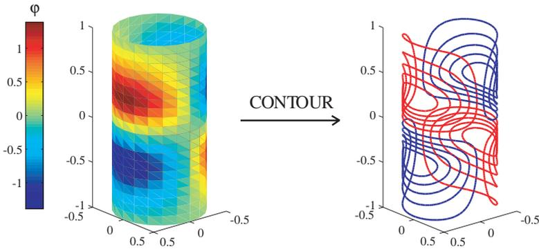
**Figure 5.** Stream function over the coil surface and wire arrangement (stream lines). Note that  $\varphi$  is normalized to unity since its scale is unimportant for contouring purposes. We choose a number of contour levels  $N_c = 10$  that are equally spaced [4] (Brideson et al. [19] proved that equally spaced contours of  $\varphi$  give an approximation to  $\mathbf{J}$ ).
