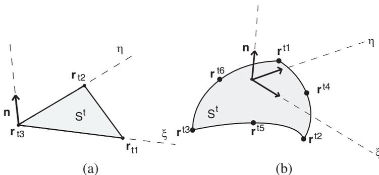
**Figure 3.** Coordinates system  $(\xi, \eta)$  for (a) flat elements and (b) quadratic curved element.
