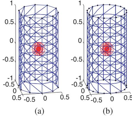
**Figure 4.** Cylinder meshed using (a) 160 flat elements (b) and using 160 quadratic curved elements. The ROI is formed from a spherical distribution of 400 points (in red) at the centre of the figure; and the nodes at the edges are marked in black.
