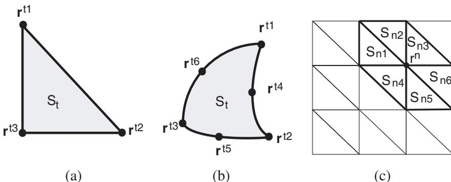
**Figure 1.** (a)  $T2N(S_t)$  for a linear flat element ( $\Lambda = 3$ ); (b)  $T2N(S_t)$  for a quadratic element ( $\Lambda = 6$ ). The  $N2T(\mathbf{r}_n)$  function relates a given node  $\mathbf{r}_n$  with the elements to which it belongs; (c) flat linear elements.
