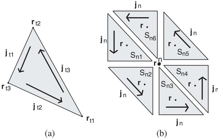
**Figure 2.** (a) Current basis vectors in one flat element; (b) current basis vector associated to the  $n$ th-node  $\mathbf{j}^n(\mathbf{r})$  (its value depends on the particular element which  $\mathbf{r}$  lies in).
