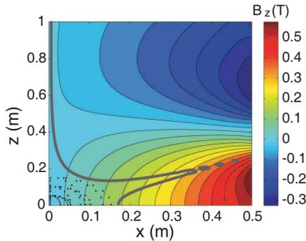
**Figure 6.** Contours of the  $B_z$  field produced by the wire arrangement Fig. 5. The grey line delineates the region where the field deviates by less than 5% from linearity. The points where the field is evaluated in the ROI are shown in black. The target field employed is  $B_z(r) = G_x x$ , where the gradient proportionality constant has been considered as  $G_x = 1 \text{ T/m}$ . The current intensity carried by the coil to produced this field is then  $I = 24.53 \text{ kA}$ .
