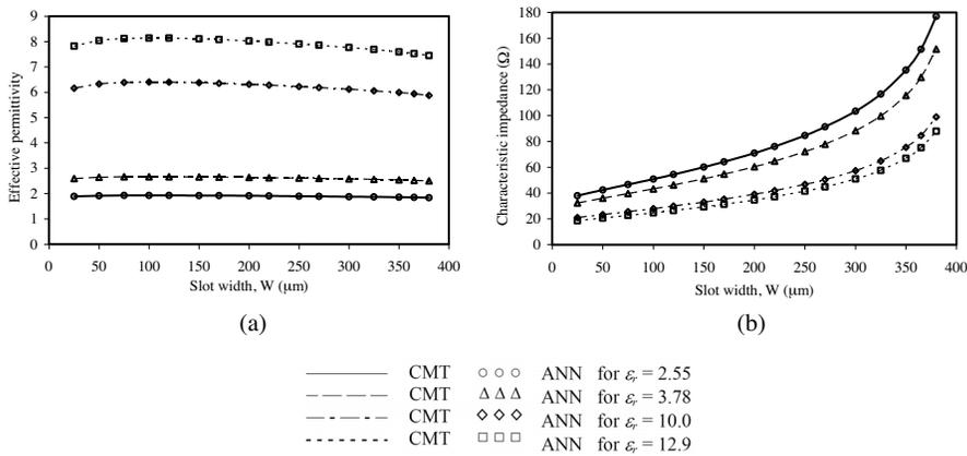
**Figure 4.** Comparison of the neural model and CMT [4] results for the characteristic parameters of CSMLs with  $h_1 = 3 \text{ mm}$ ,  $h_2 = 400 \text{ }\mu\text{m}$ ,  $b = 400 \text{ }\mu\text{m}$ , and  $\epsilon_r = 2.55, 3.78, 10,$  and  $12.9$ . (a) Effective permittivity and (b) Characteristic impedance.
