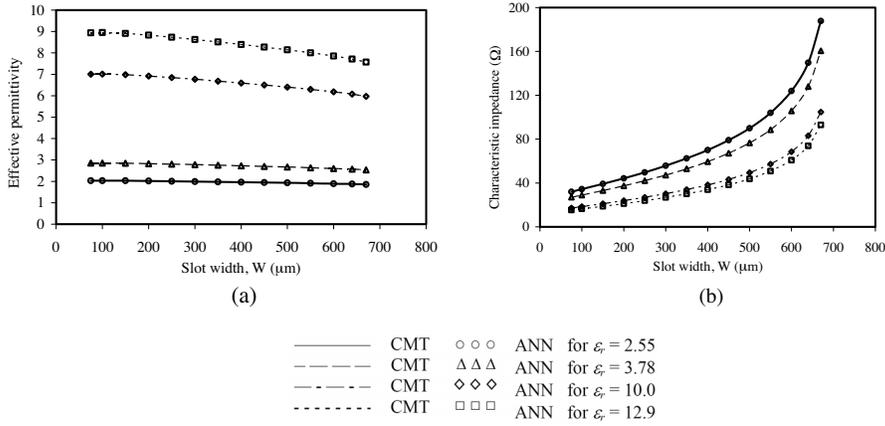
**Figure 3.** Comparison of the neural model and CMT [4] results for the characteristic parameters of ESMLs with  $h_1 = 3 \text{ mm}$ ,  $h_2 = 400 \text{ }\mu\text{m}$ ,  $b = 692.82 \text{ }\mu\text{m}$ , and  $\epsilon_r = 2.55, 3.78, 10,$  and  $12.9$ . (a) Effective permittivity and (b) Characteristic impedance.
