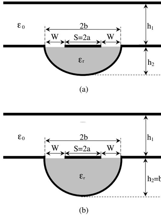
**Figure 1.** Microshield lines, (a) ESML and (b) CMSL.
