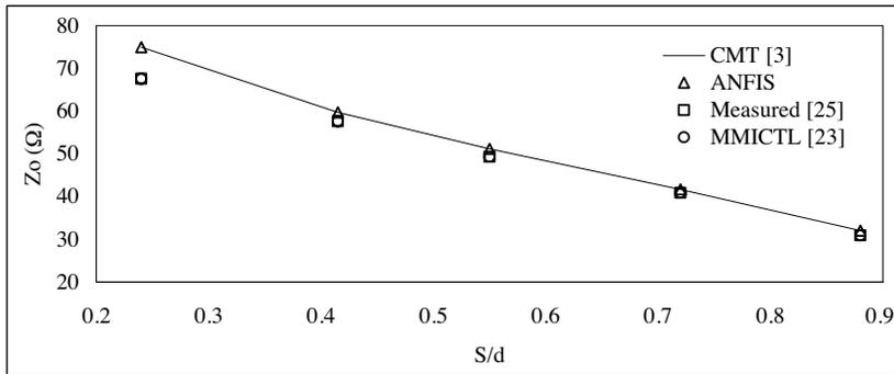
(b)  $d = 1000 \mu\text{m}$ ,  $h = 640 \mu\text{m}$ , and  $\epsilon_r = 9.7$
