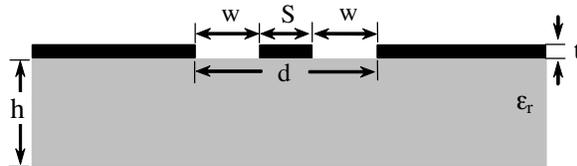
**Figure 1.** Cross-section of a CCPW.
