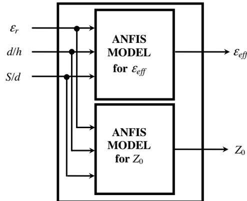
**Figure 3.** The structure of proposed ANFIS model.
