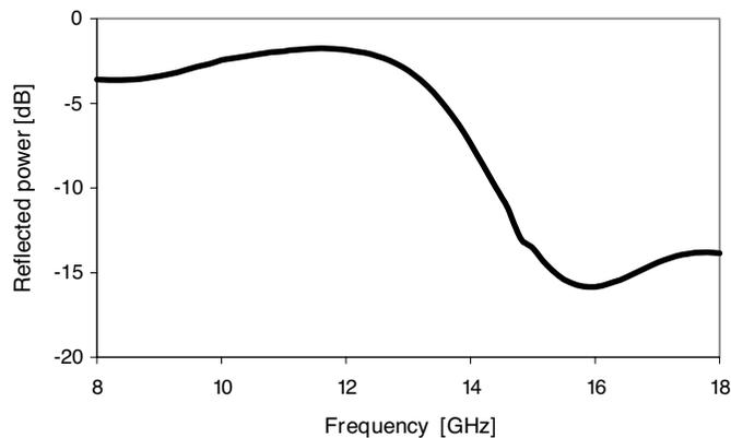
**Figure 3.** Measured reflected power in dB from the absorbing mechanism shown in Figure 2 at  $x = 4.7$  mm.
