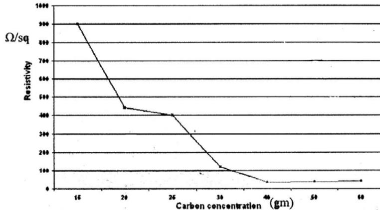
**Figure 1.** Effect of carbon concentration on the resistivity value obtained from plain woven fabric.
