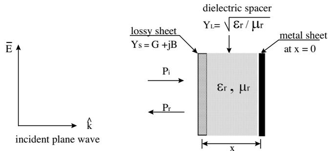
**Figure 2.** Configuration of Salisbury screen as single layer absorbing mechanism.
