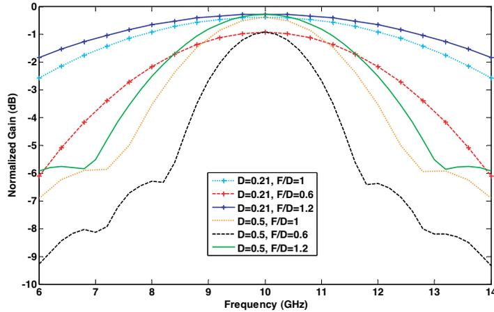
**Figure 6.** Variation of the normalized gain of the simulated reflectarrays with frequency, for array diameters of 0.21 and 0.5 m, and the shown  $F/D$  ratios.
