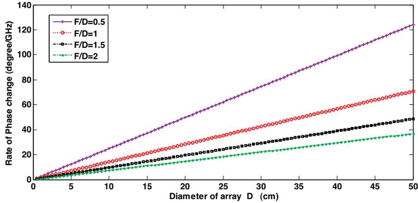
**Figure 4.** Variation of  $d\Phi/df$  against array diameter at various  $F/D$  ratios.
