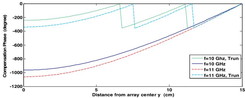
**Figure 5.** Compensation phase variation along array radius, and the truncated phase at two frequencies of operation, array diameter = 0.3 m, and  $F/D = 1/3$ .
