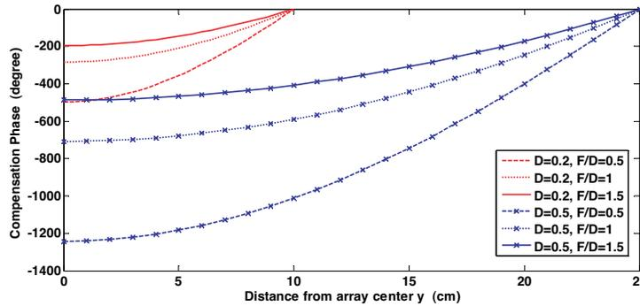
**Figure 2.** Phase variation with distance from centre of array at various  $F/D$  ratios, for two array sizes of 0.2 m and 0.5 m, at frequency of 10 GHz.
