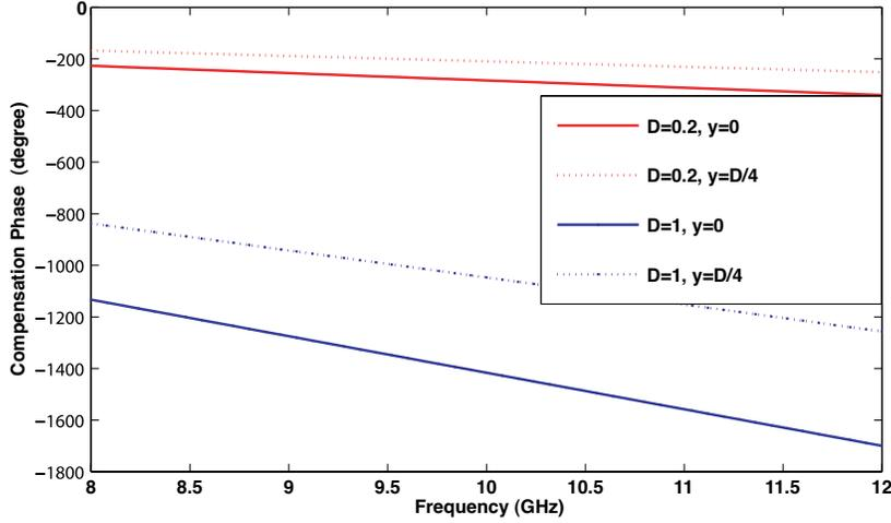
**Figure 3.** Phase variation with frequency at  $y = 0$  and  $y = D/4$ , for array sizes of 0.2 m and 1 m, for  $F/D = 1$ .
