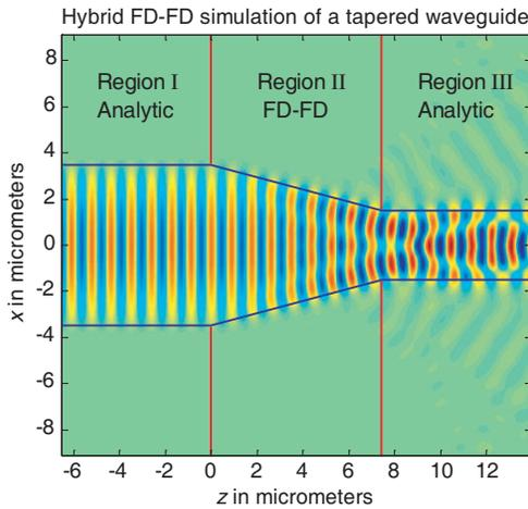
**Figure 1.** Illustration of the hybrid FD-FD method applied to a quasi-adiabatic tapered waveguide device. The field  $E_y(x, z)$  is excited by A TE-polarized fundamental mode incident wave. This ideal 2-D device is made of a glass core with an air cladding.
