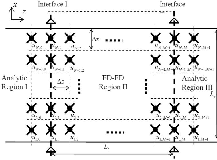
**Figure 2.** The Layout of the grid points in the FD-FD region shows a total of  $N \times M$  unknowns in the  $L_z$  by  $L_x$  domain. The first and the last column of grid vectors are auxiliary variables located in the analytical regions.
