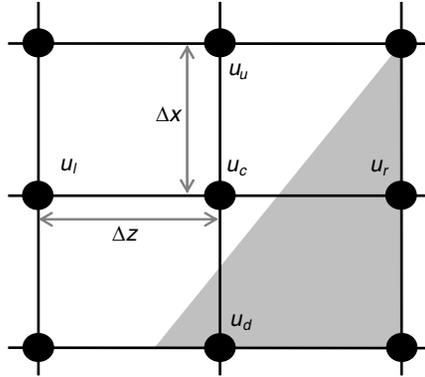
**Figure 3.** FD-FD TE grid points near a material interface.
