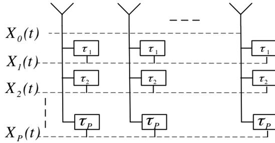
**Figure 1.** The received signal with delayed output.
