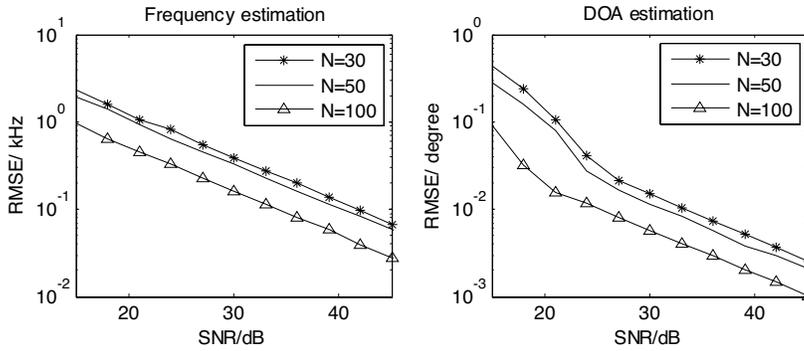
**Figure 5.** Angle-frequency estimation with different snapshot  $N$ .
