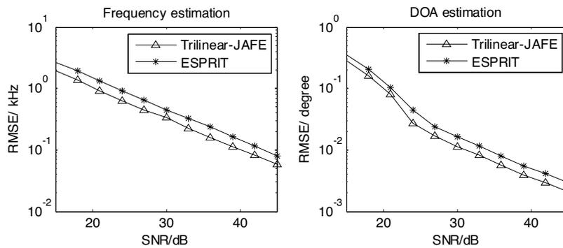
**Figure 3.** Angle-frequency estimation performance comparison.
