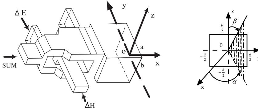
**Figure 1.** The coordinate system and the geometry of the rectangular horn antenna, where  $a = 2.1\lambda$ ,  $b = 1.9\lambda$ ,  $\lambda$  is a wavelength,  $\alpha$  and  $\beta$  denote an azimuth angle and an elevation angle respectively.
