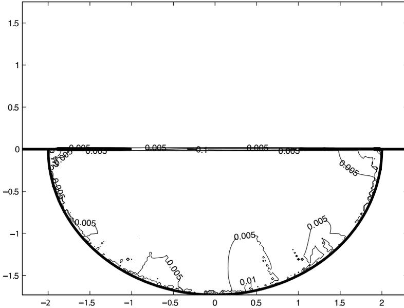
**Figure 10.** Contour plot of  $|H_z^{I.E.} - H_z^{analytic}|$  for the results shown in Fig. 9. No contour lines are shown for  $y > 0$  because the differences are negligible.
