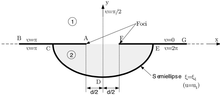
**Figure 1.** Semielliptical channel-backed slot.
