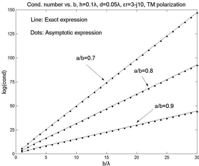
**Figure 7.** Matrix condition number (both exact and asymptotic expressions) as a function of the scatterer radius  $b$ , for  $h_\lambda = 0.1$ ,  $d = 0.05\lambda$ ,  $\epsilon_r = 3 - j10$ , various values of the ratio  $a/b$  and TM incidence.
