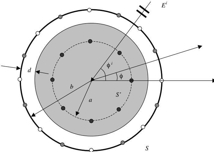
**Figure 1.** Geometry of the problem. Black, white and gray bullets represent Auxiliary Sources (AS's), Collocation Points (CP's) and Midpoints (MP's) respectively. The gray disk corresponds to the PEC cylinder, coated by the dielectric layer, colored white.
