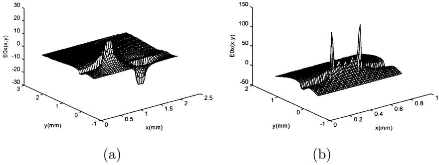
**Figure 2.**  $x$ -component of voltage sources. (a) Coplanar wave guide ( $w = 0.9$  mm,  $s = 0.5$  mm, substrate thickness  $h = 0.635$  mm,  $\epsilon_r = 9.9$ , housing WR28,  $F = 15$  GHz) (b) Finline (gap  $w = 0.3$  mm, substrate thickness  $h = 0.11$  mm,  $\epsilon_r = 3.75$ ,  $F = 80$  GHz).
