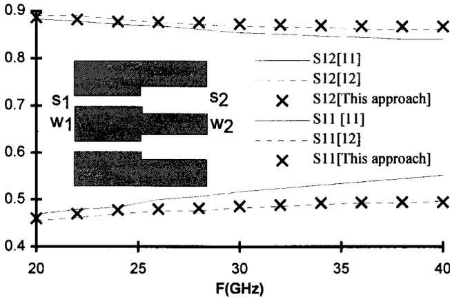
**Figure 6.** *S*-parameters of a simple step discontinuity in a coplanar wave guide; Dimensions:  $s_1 = 0.1$  mm,  $s_2 = 0.4$  mm,  $w_1 = 0.4$  mm,  $w_2 = 0.1$  mm, dielectric constant  $\epsilon = 9.6$  and thickness  $h = 0.254$  mm.
