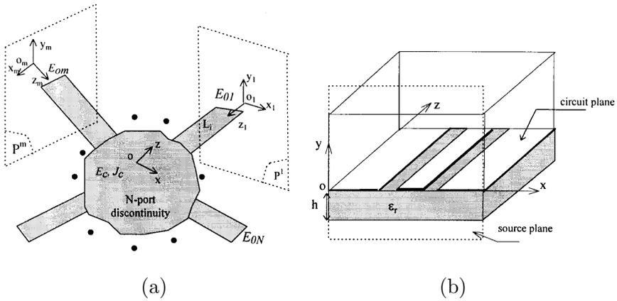
**Figure 1.** (a) Schematic of a multiport discontinuity. (b) transition source-line (case of a CPW)
