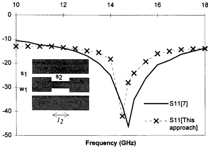
**Figure 5.**  $S_{11}$ -parameter of a double step discontinuity in a coplanar circuit; Dimensions:  $s_1 = 0.2$  mm,  $w_1 = 0.5$  mm,  $s_2 = 0.35$  mm,  $l_2 = 4.36$  mm,  $h = 0.635$  mm,  $\epsilon_r = 9.9$ , housing WR28.
