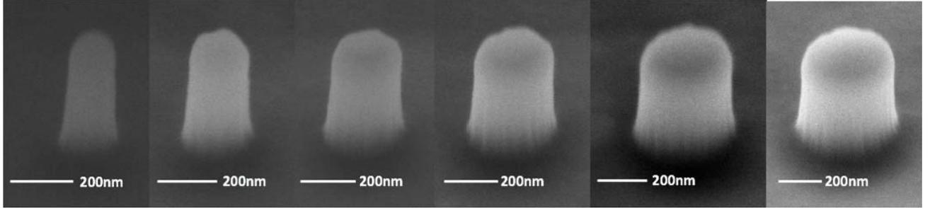
**Figure 1.**  $45^\circ$  tilted SEM images of single nanowires. (diameter (from left to right): 150, 200, 250, 300, 350, and 400 nm).
