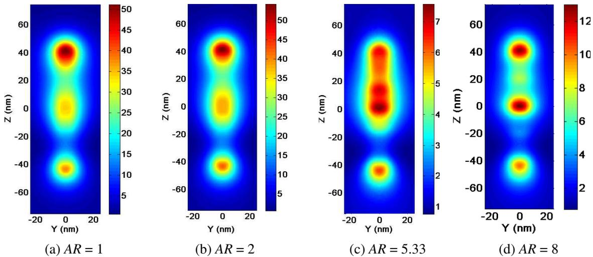
**Figure 6.** Near-field intensity distribution calculated 5 nm above the rod, at the resonance of the second mode ( $\lambda = 440$  nm). Calculations performed using GDT with meshes of different aspect ratios as indicated in the figures.
