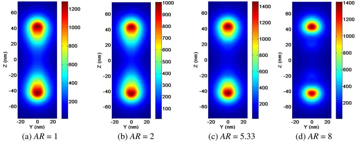
**Figure 3.** Near-field intensity distribution calculated 5 nm above the rod surface at the wavelength  $\lambda = 682$  nm. The hemispherical caps are discretized with cubic cells of length 2.5 nm whereas the central part is discretized with rectangular parallelepipeds of dimensions  $a \times b \times c$  with  $b = c = 2.5$  nm and different aspect ratio  $AR = a/b$ .  $a$  varies from  $a = 2.5$  nm ( $AR = 1$ ) to  $a = 20$  nm ( $AR = 8$ ). Calculations performed using GDT.
