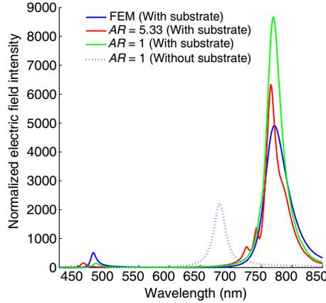
**Figure 8.** Near-field intensity spectrum calculated at one silver rod extremity (point  $P$ , located 4 nm away from the silver rod tip). FEM: Finite Element Method.  $AR = 5.33$  and  $AR = 1$ : GDT with cell aspect ratio  $a/b = 5.33$  and  $a/b = 1$  (with  $b = c = 1.6$  nm), respectively. The rod is on a glass substrate of dielectric constant  $\epsilon_{sub} = 2.25$ . The dotted curve represents the spectrum in absence of the substrate for comparison.
