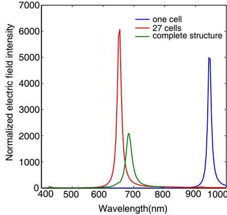
**Figure 4.** Electric field intensity calculated 4 nm away from a single cell (blue curve, ‘one cell’), a  $3 \times 3 \times 3$  cells object (red curve ‘27 cells’) and the complete structure (green curve). The cell aspect ratio is  $AR = 5.33$ .
