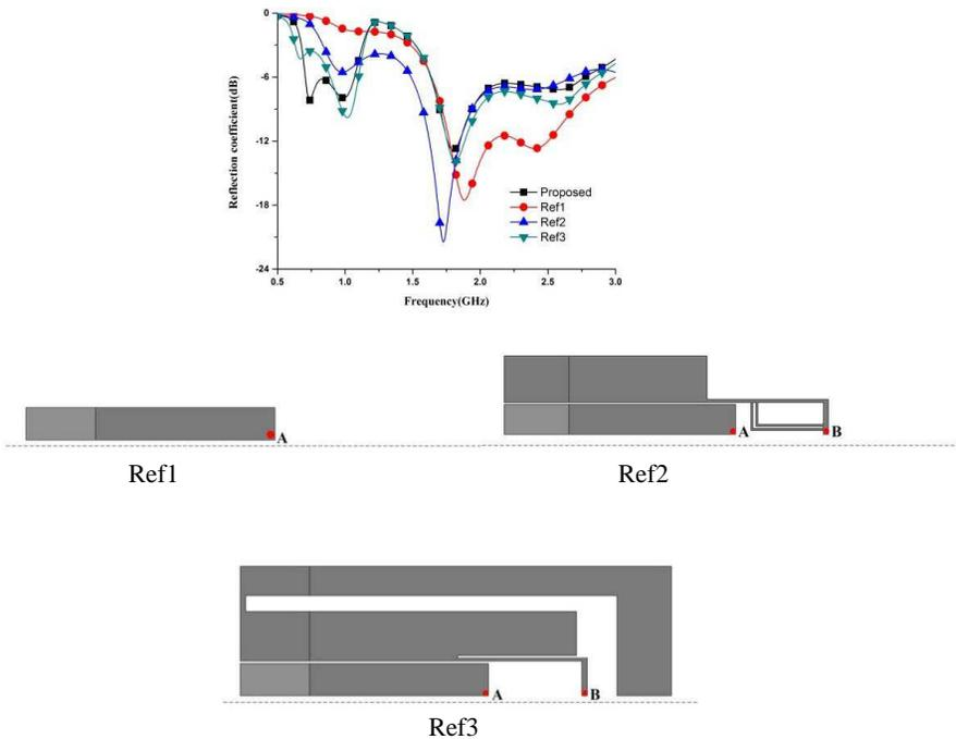
**Figure 4.** Simulated reflection coefficient of different antenna variations. Ref1. The case with the driven monopole only; Ref2. The case with the coupled loop antenna; Ref3. The case without two adding branch strips.
