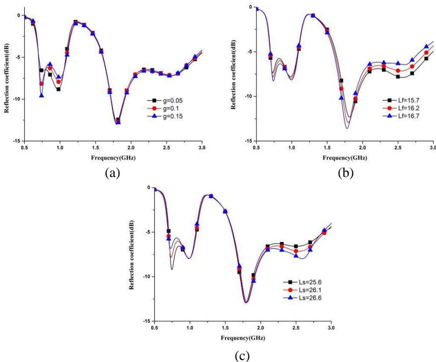
**Figure 5.** Simulated reflection coefficient of the proposed antenna as a function of (a) the width of gap, (b) the length  $L_f$ , and (c) the length  $L_s$ . Other dimensions are the same as given in Figure 1.
