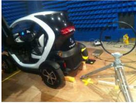
**Figure 3.** ROHDE & SCHWARZ loop antenna used in the measurements.
