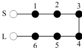
**Figure 7.** The topology of the six-pole Chebyshev filter.
