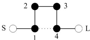
**Figure 2.** The topology of the fourth-order cross-coupled filter.
