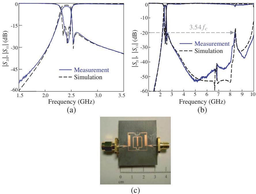
**Figure 9.** Simulated and measured responses of the first proposed triple-mode filter in (a) 1.5 ~ 3.5 GHz and (b) 1 ~ 10 GHz. (c) Photograph of the measured circuit. All sizes are given in Fig. 8.
