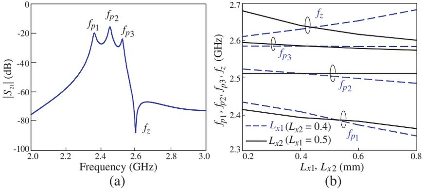
**Figure 4.** (a) Transmission response of Fig. 3(a) with  $L_e = 0$ . (b) Resonant frequencies and transmission zero position versus  $L_{x1}$  and  $L_{x2}$ .  $W_{c1} = W_{c2} = 0.2$  mm, radius of via hole  $r = 0.2$  mm. Parameters:  $2L_1 = 9.3$ ,  $L_2 = 10.75$ ,  $L_3 = 16.3$ ,  $L_s = 6.55$ ,  $W_1 = 1.8$ ,  $W_2 = 0.2$ ,  $W_3 = 0.5$ ,  $W_s = 1.1$ ,  $W_{c1} = W_{c2} = W_e = 0.2$ ,  $L_{x1} = 0.6$ ,  $L_{x2} = 0.4$ . All sizes are in mm.
