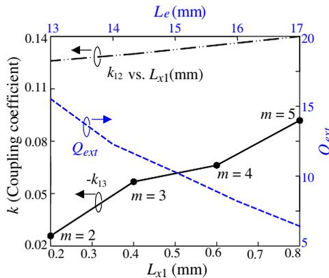
Figure 11. Design graphs: change of  $k_{12} = k_{23}$  versus  $L_{x1}$  with  $m = 4$  and  $W_{c1} = 0.2$  mm, variation of  $-k_{13}$  against  $m$  with  $L_{x1} = 0.35$  mm and  $W_{c2} = 0.2$  mm, and dependence of  $Q_{ext}$  on  $L_e$ . All sizes are given in Fig. 5.
