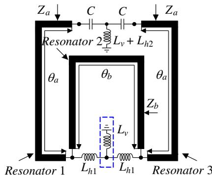
**Figure 2.** Generic structure of the proposed triple-mode resonator.
