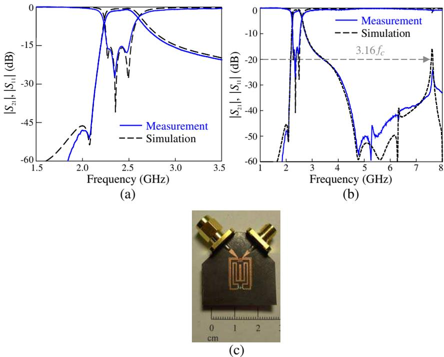
**Figure 12.** Performance of the triple-mode resonator bandpass filter with capacitive cross coupling. (a) 1.5 ~ 3.5 GHz and (b) 1 ~ 8 GHz. (c) Photograph of the measured circuit. All circuit geometric parameters are in Fig. 5.
