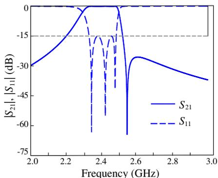
Figure 7. Frequency response synthesized by coupling matrix (6).
