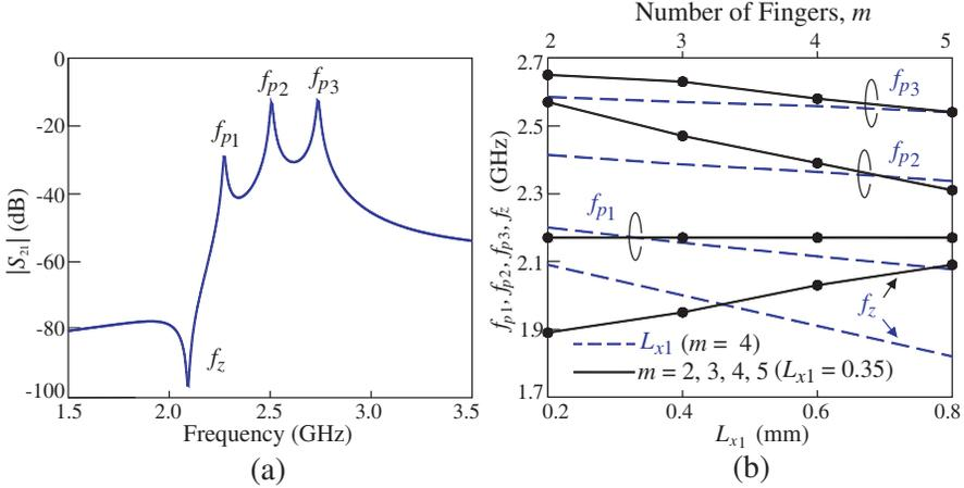
**Figure 6.** (a) Transmission response of Fig. 5 with  $L_e = 0$ . (b) Resonant frequencies and transmission zero frequency versus  $L_{x1}$  and number of interdigital fingers  $m$ . Substrate:  $\epsilon_r = 2.2$ , thickness  $h = 0.508$  mm.
