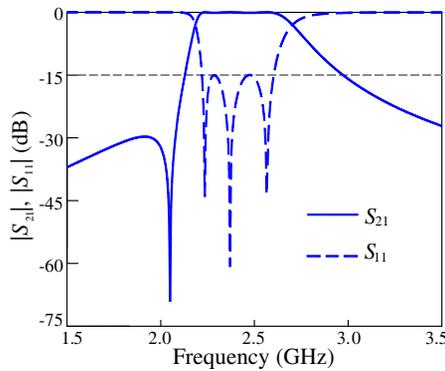
Figure 10. Frequency response synthesized by coupling matrix (9).
