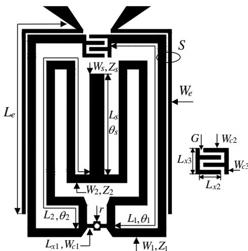
**Figure 5.** Layout of the triple-mode resonator with capacitive coupling.  $L_1 = 18$ ,  $L_2 = 22.6$ ,  $L_s = 6.4$ ,  $W_1 = W_2 = 0.5$ ,  $W_s = 0.9$ ,  $W_{c1} = 0.2$ ,  $L_{x1} = 0.35$ ,  $W_{c2} = W_{c3} = 0.2$ ,  $L_{x2} = 1.05$ ,  $L_{x3} = 1.6$ ,  $G = 0.15$ ,  $r = W_e = 0.2$ ,  $L_e = 15.5$ . All sizes in mm.
