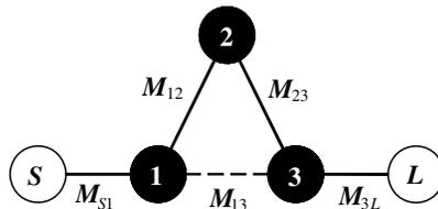
**Figure 1.** Coupling scheme of a trisection bandpass filter.
