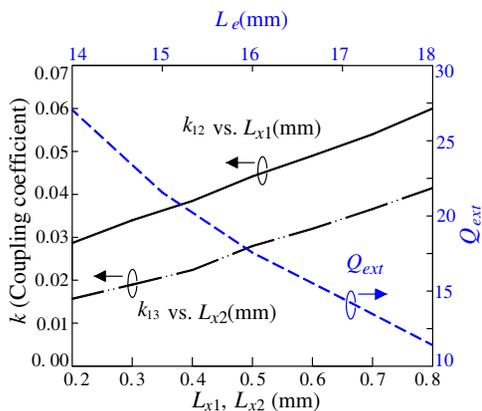
Figure 8. Design graphs: change of  $k_{12} = k_{23}$  versus  $L_{x1}$  with  $L_{x2} = 0.55$  mm, variation of  $k_{13}$  against  $L_{x2}$  with  $L_{x1} = 0.5$  mm and dependence of  $Q_{ext}$  on  $L_e$ . Parameters:  $2L_1 = 9.3$ ,  $L_2 = 10.75$ ,  $L_3 = 16.3$ ,  $L_s = 7.55$ ,  $W_1 = 1.8$ ,  $W_2 = 0.2$ ,  $W_3 = 0.5$ ,  $W_s = 1.1$ ,  $W_{c1} = W_{c2} = W_e = 0.2$ ,  $L_{x1} = 0.5$ ,  $L_{x2} = 0.55$ ,  $S = 0.15$ ,  $r = 0.2$ ,  $L_e = 16.4$ . All sizes are in mm.
