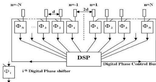
**Figure 7.** Centrosymmetric antenna array using digital phase shifters.
