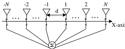
**Figure 3.** Centro-symmetric thinned linear antenna array.
