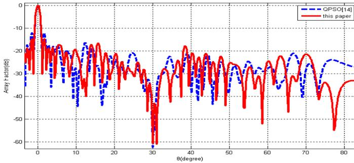
**Figure 8.** The optimized array pattern with minimum PSLL and null control (solid). 100 elements, null positions are  $30^\circ$  and  $31^\circ$ , PSLL =  $-14.7$  dB, HPBW =  $0.8^\circ$ , directivity =  $24.2$  dB.
